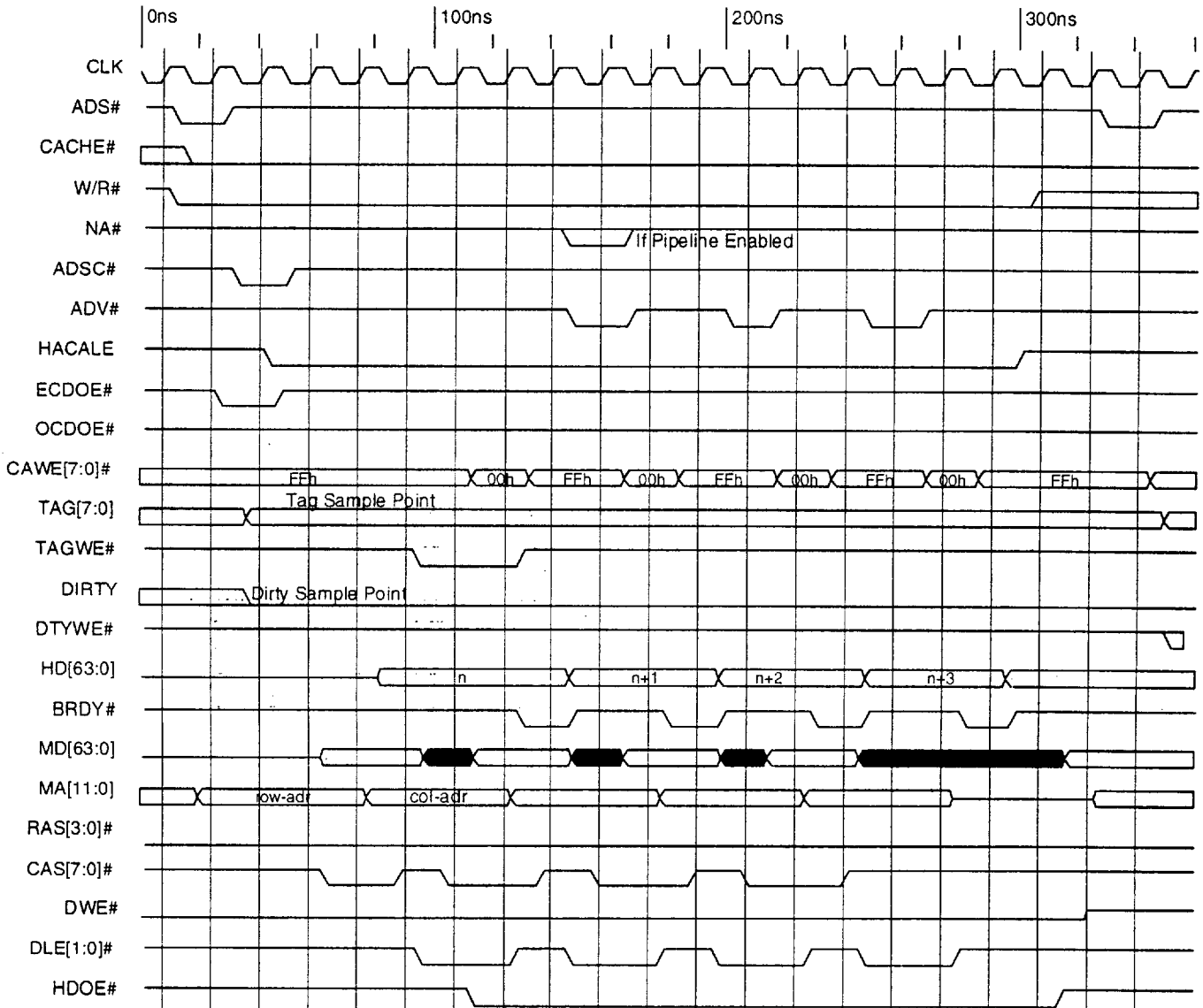
Figure 4-11 L2 Cache Read Miss Clean Burst of 8-3-3-3 (Linefill Cycle) - Sync SRAMs
