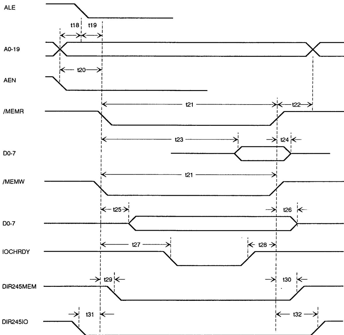
**AC Specifications****16 Bit I/O Bus Cycles**
