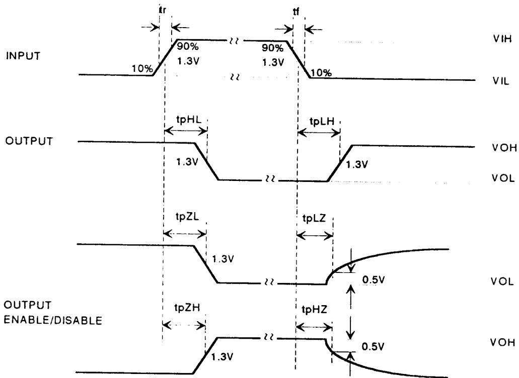
$V_{IH} = 3 \text{ V}$ ,  $V_{IL} = 0$ ,  $t_r < 10 \text{ ns}$ ,  $t_f < 5 \text{ ns}$
