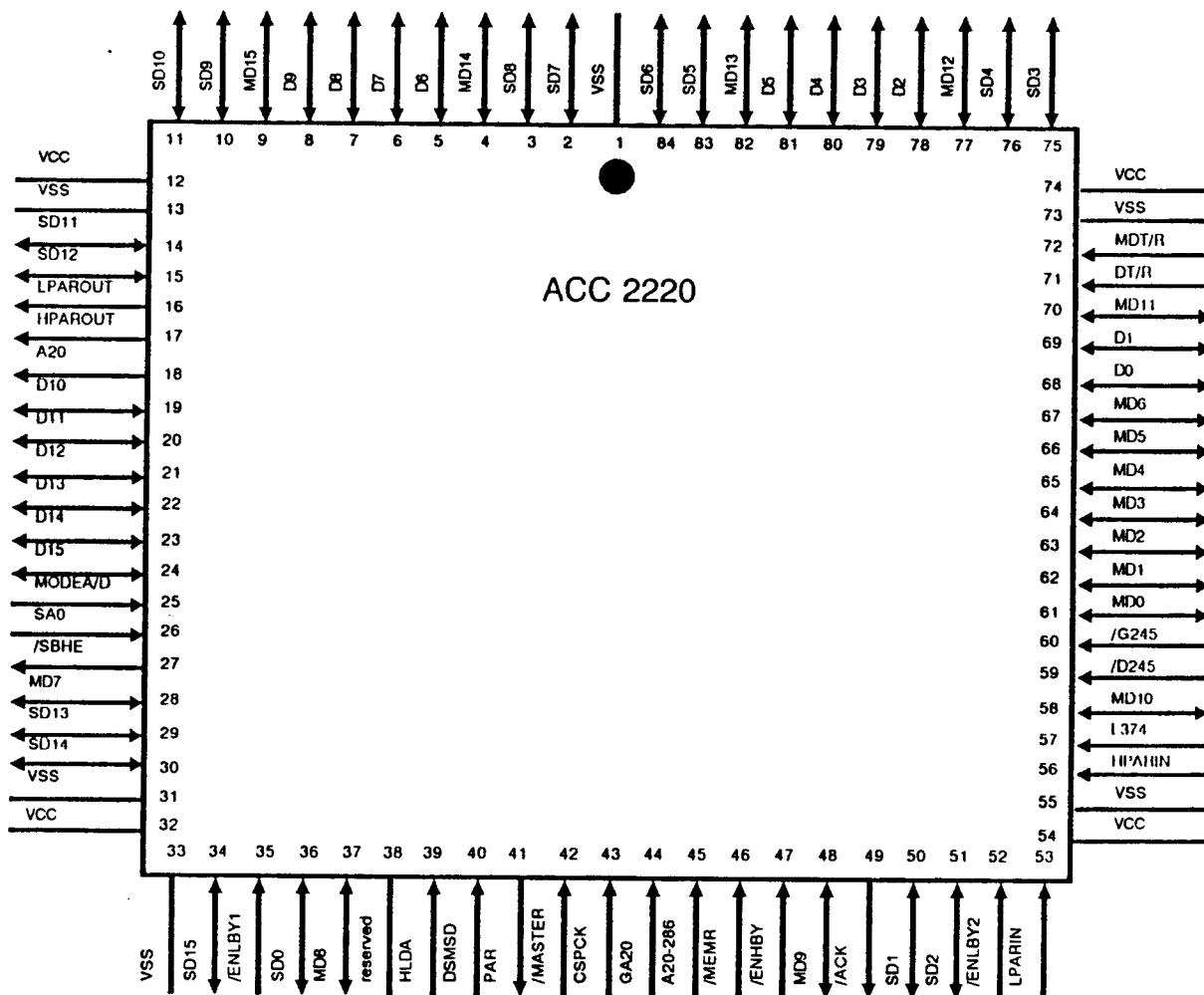
Pin Diagram (ACC 2220 Address Buffer Mode)
