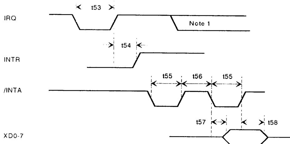
Note 1 IRQ must remain active until the first /INTA pulse.
