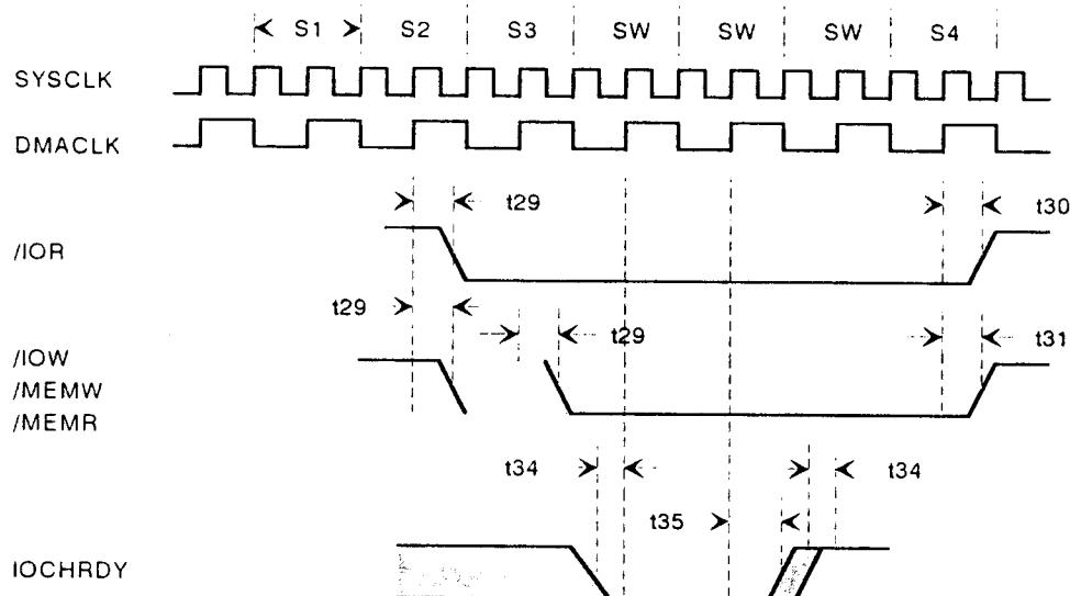
The first wait state is inserted by the internal circuitry of the ACC 2000 for all DMA cycles.
