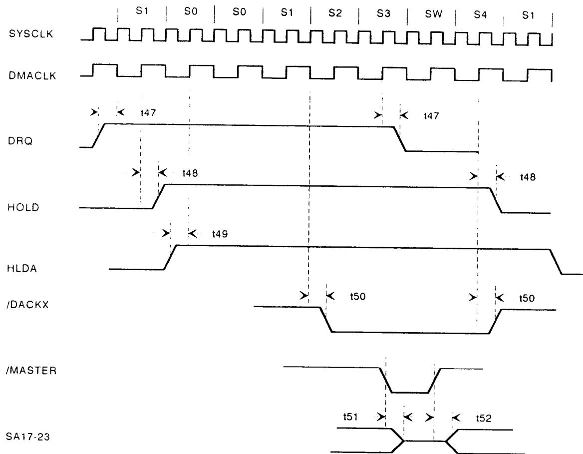
Note: A new bus master must be programmed in Cascade mode.
