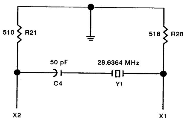
Figure 1 Example Crystal Oscillator Circuit using the ACC 1000
