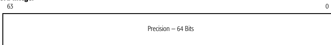
Figure 8. Integer Data Registers
