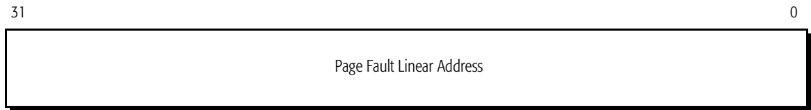
Figure 23. Control Register 2 (CR2)
