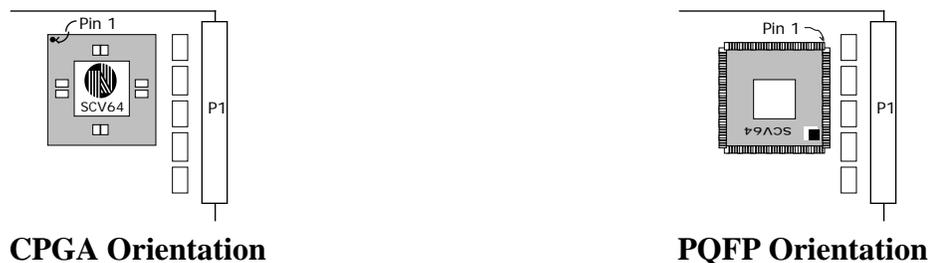
**Figure 2: Orientation of the SCV64 (CPGA and PQFP) to Minimize Distance to the Connector**
