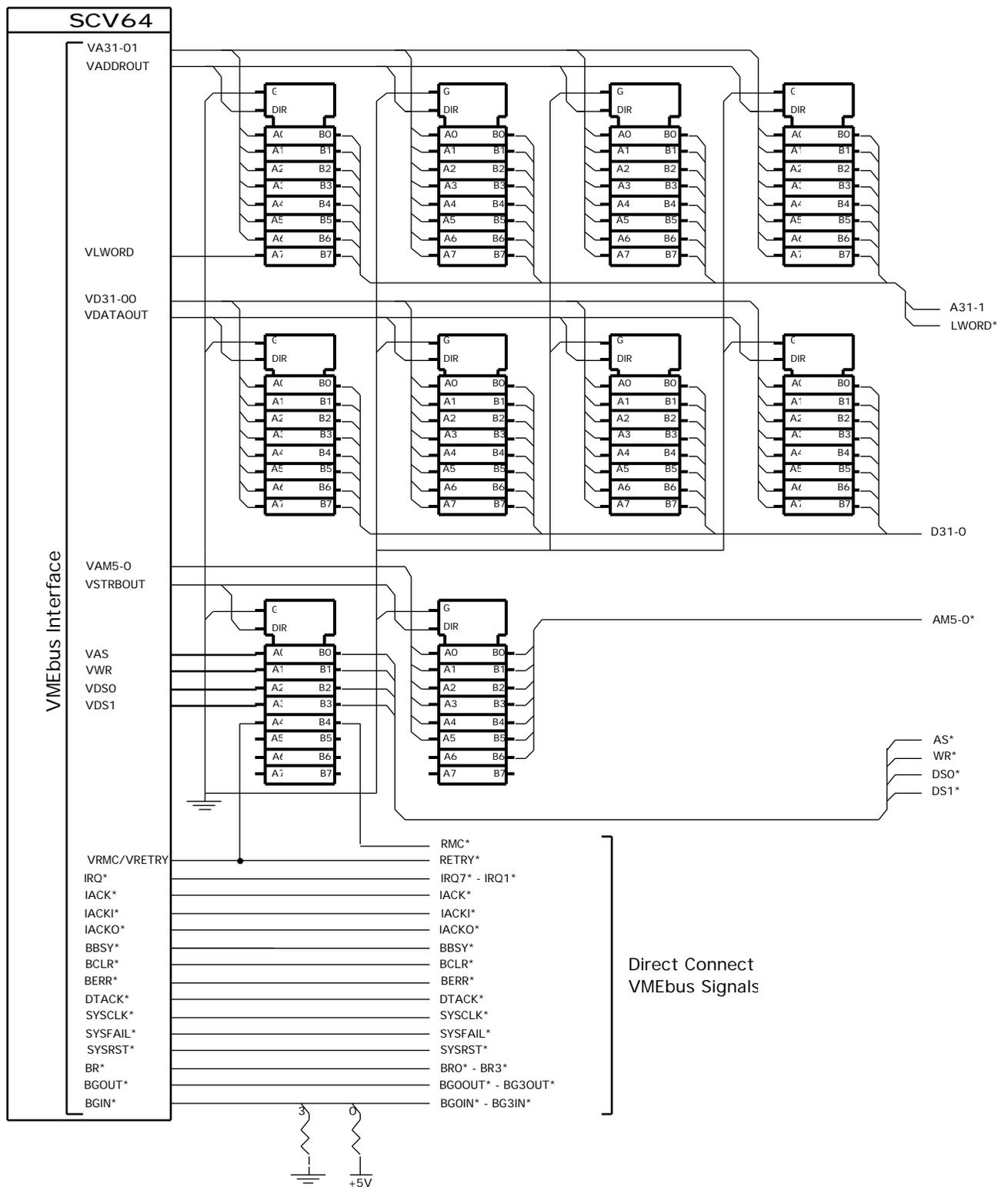
Figure 1: SCV64 Interface to VMEbus
