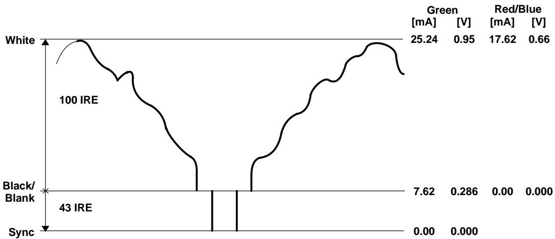
Figure 10. 0-IRE, 8-Bit Composite Video Output
