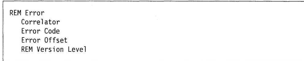
Figure 15-6. REM Error Frame
