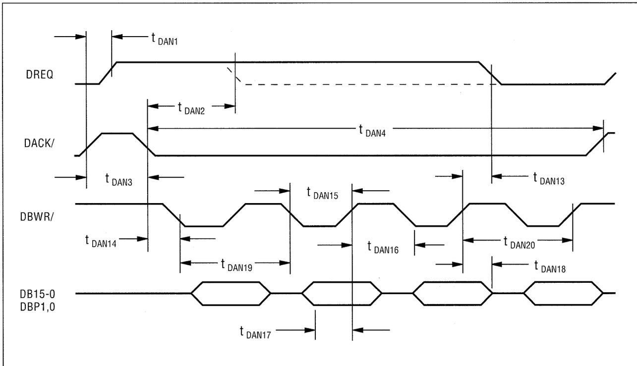
**Burst Mode DMA Interface, Nonbyte Control**
