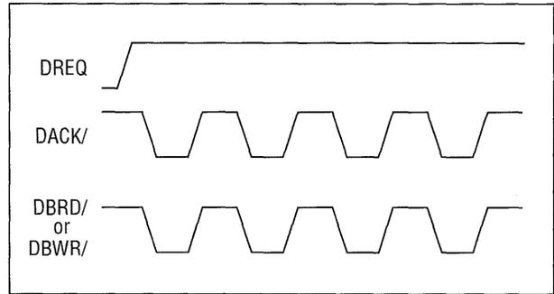
*Normal DMA Mode* illustrates the case where the threshold is always exceeded. This is typical of a DMA interface that is slower than the SCSI device to which the system is connected.
