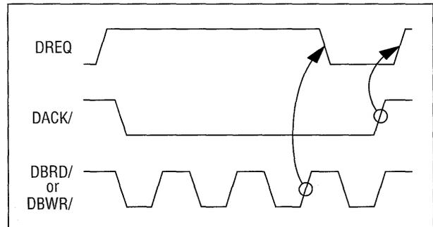
This regular surrendering of the DMA channel has two benefits for two common DMA interface problems. For DMA controllers that do not recognize higher priority requests until the current device finishes, the ASC can
