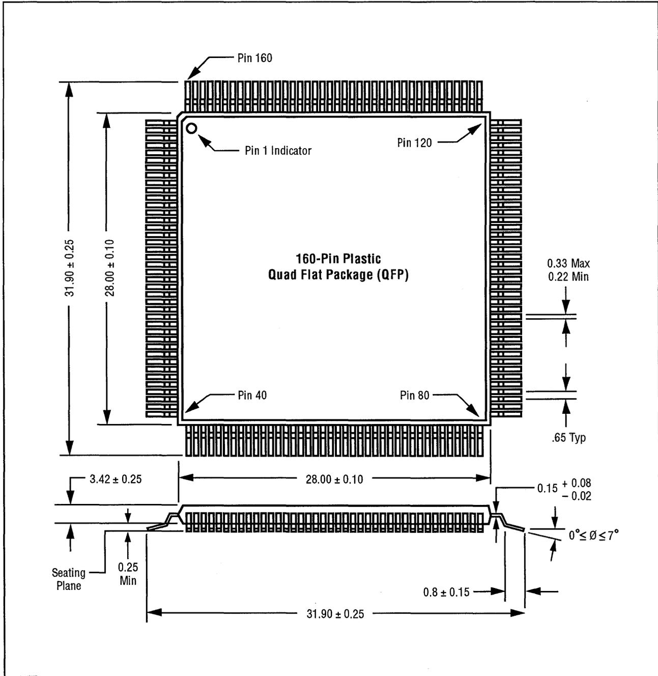
**Note:** All dimensions are in millimeters. This package is known as a Metric QFP, and should not be confused with the similar JEDEC QFP.
