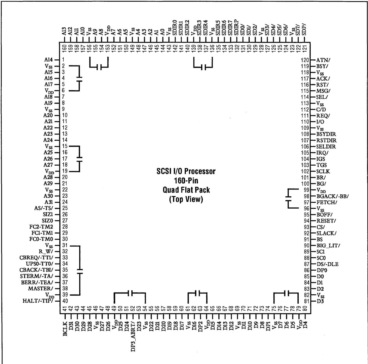
**Note:** The decoupling capacitor arrangement shown above is recommended to maximize the benefits of the internal split ground system. Capacitor values between 0.01 and 0.1  $\mu\text{F}$  should provide adequate noise isolation. Because of the number of high current drivers on the 53C710, a multilayer PC board with power & ground planes is required.
