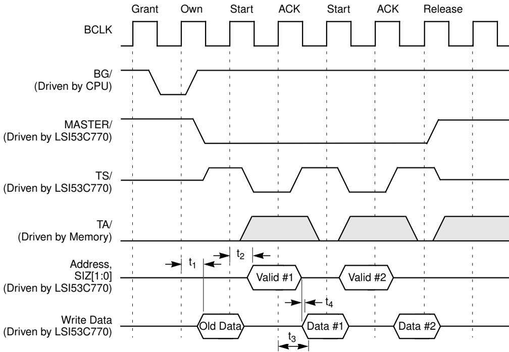
**Figure 6.27 Mux Mode Write Cycle (Cache Line Burst)**
