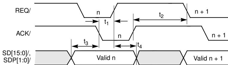
**Table 6.41 Target Asynchronous Receive Timing**
