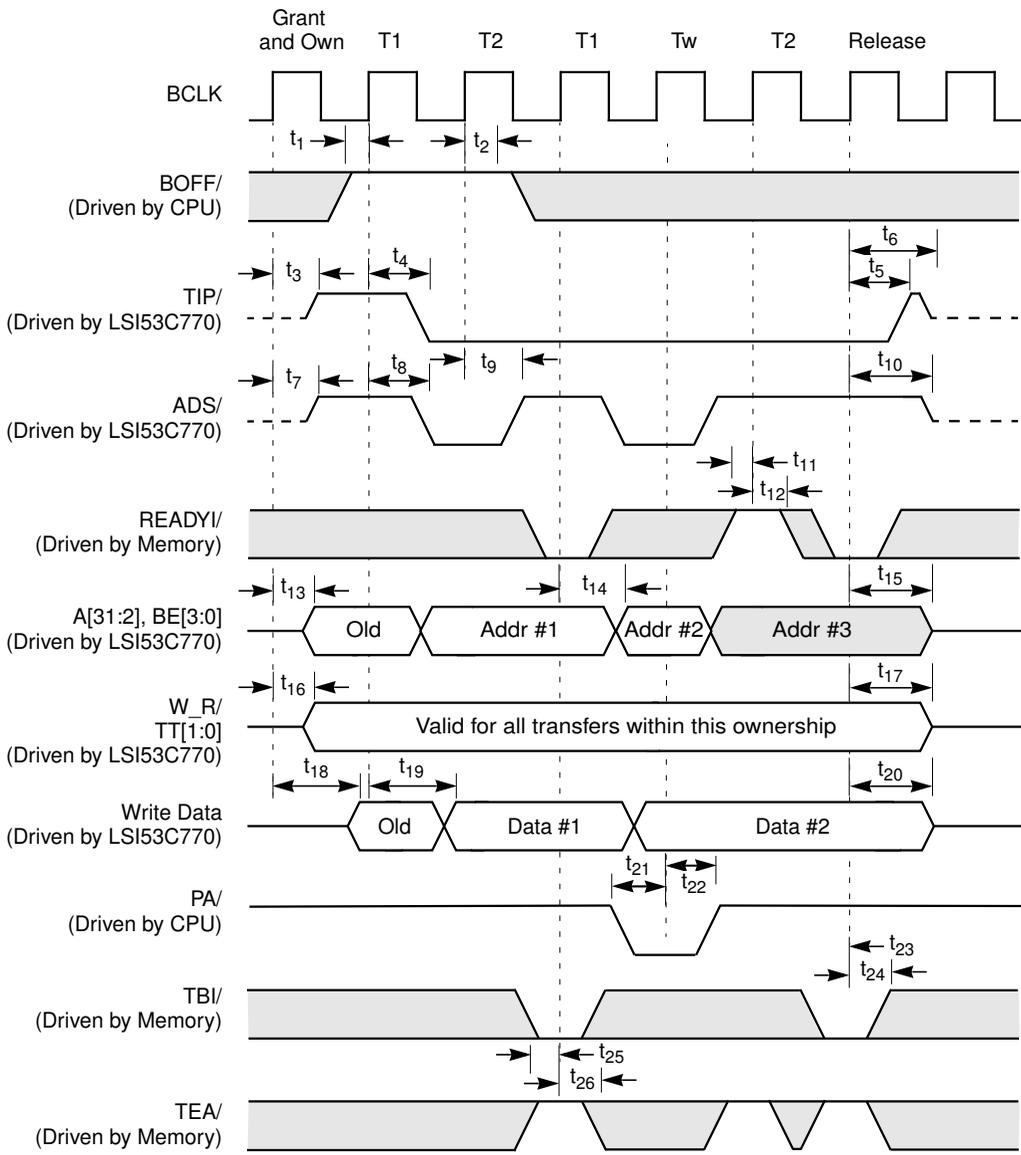
Note: This diagram shows two back-to-back transfers for a burst size of two.
