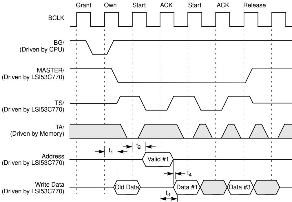
**Table 6.29 Bus Mode 2 Mux Mode Write Timing**
