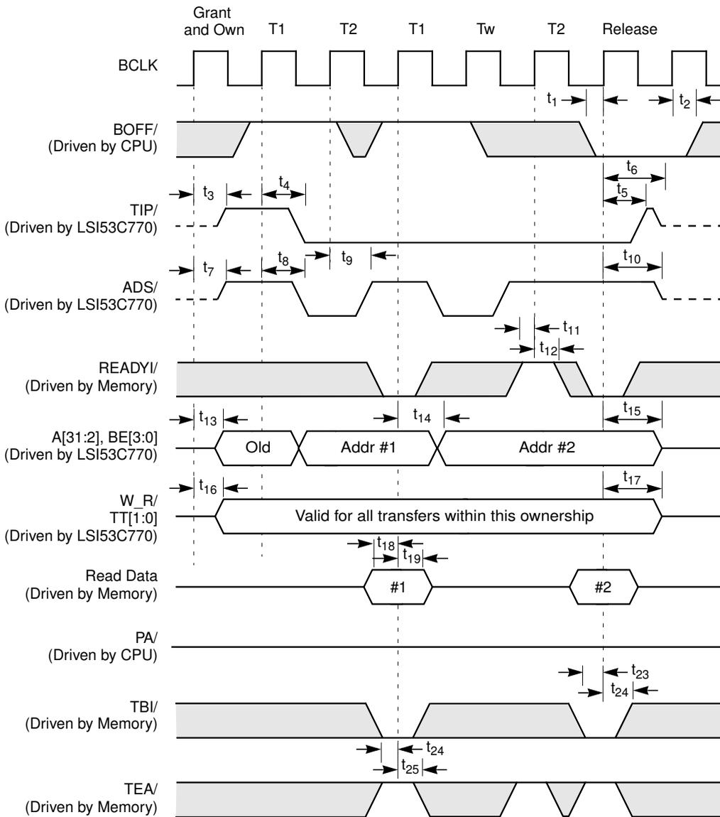
Note: This diagram shows two back-to-back cycles for a burst size of two.
