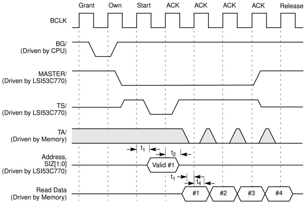
**Table 6.28 Bus Mode 2 Mux Mode Read Timing**
