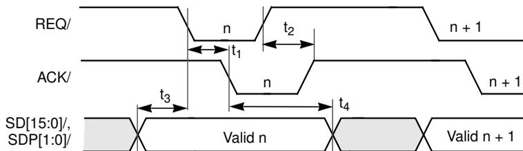
**Table 6.39 Initiator Asynchronous Receive Timing**
