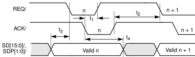
**Table 6.40 Target Asynchronous Send Timing**
