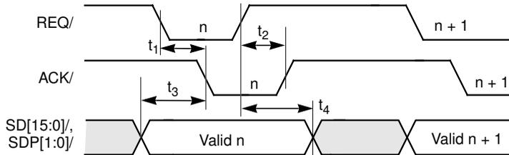
**Table 6.38 Initiator Asynchronous Send Timing**
