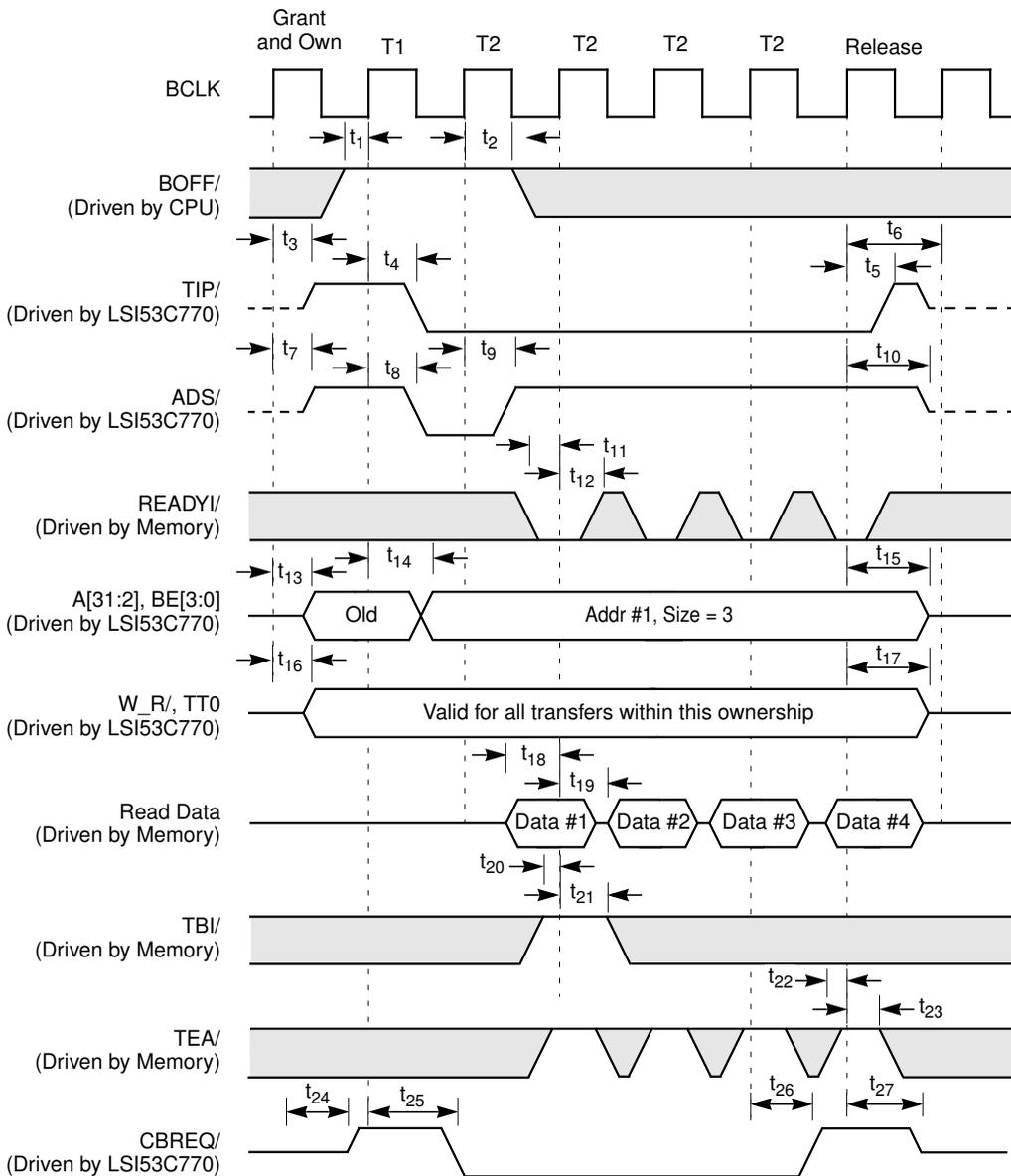
Note: This diagram shows one cache line burst of four.
