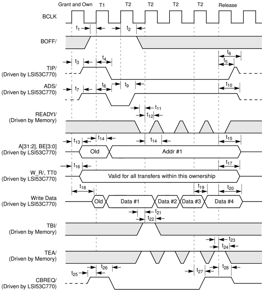
Note: This diagram shows one cache line burst of four.
