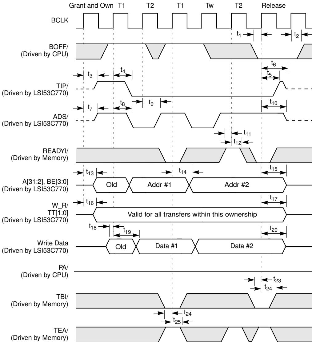
Note: This diagram shows two back-to-back transfers for a transfer size of two.
