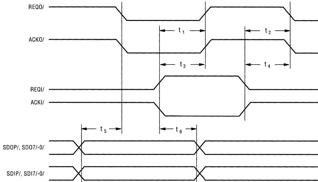
Figure 6-9. SCSI Asynchronous Input
