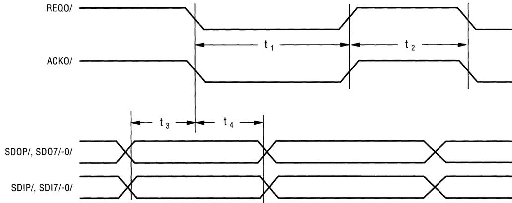
Figure 6-11. SCSI Synchronous Input
