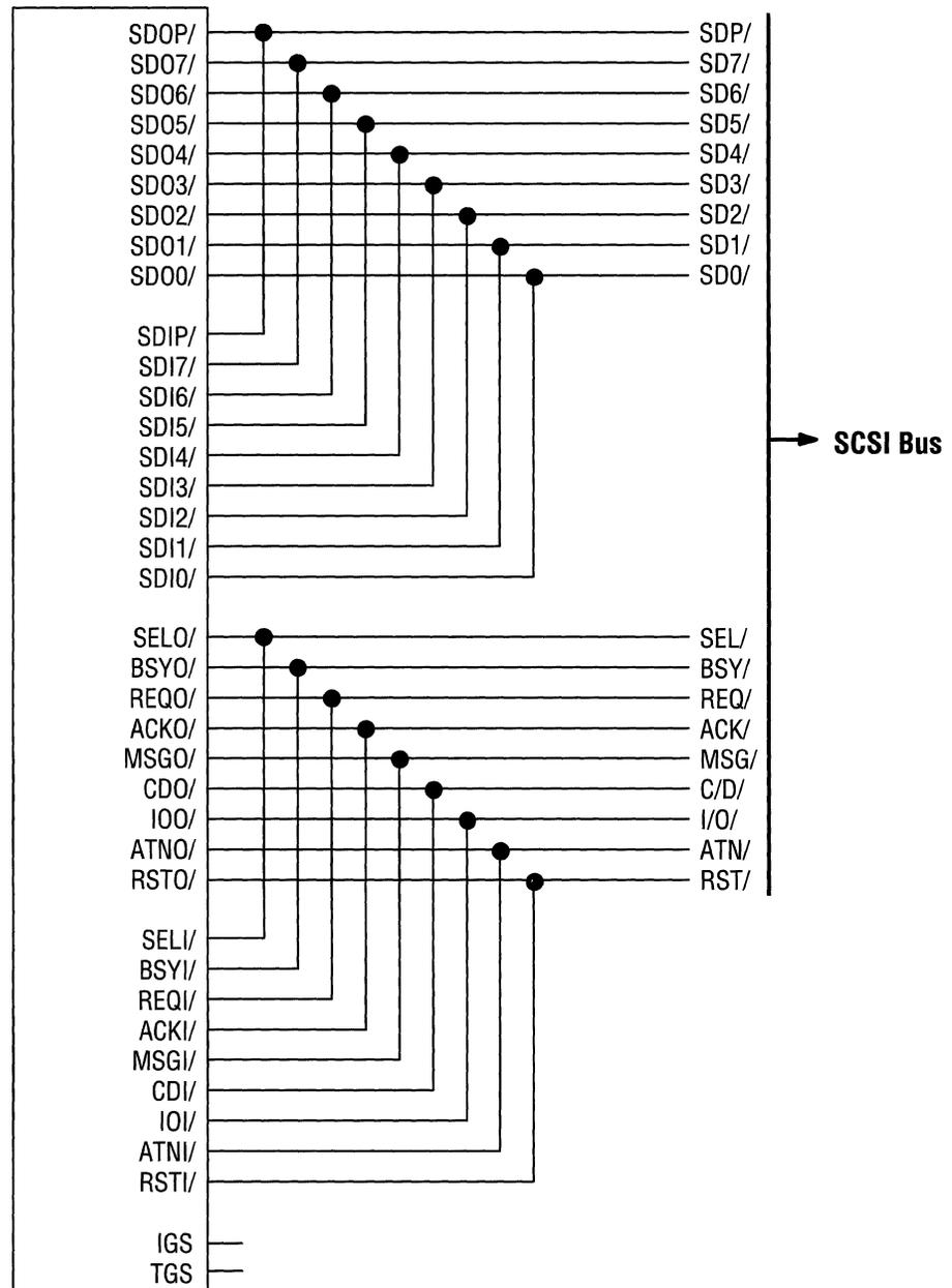
Figure C-2. NCR 53CF90A, 53CF90B Differential SCSI Bus Interface
