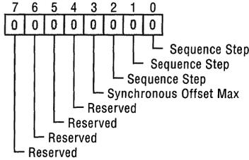
Synchronous Transfer Period Register W (06h)
