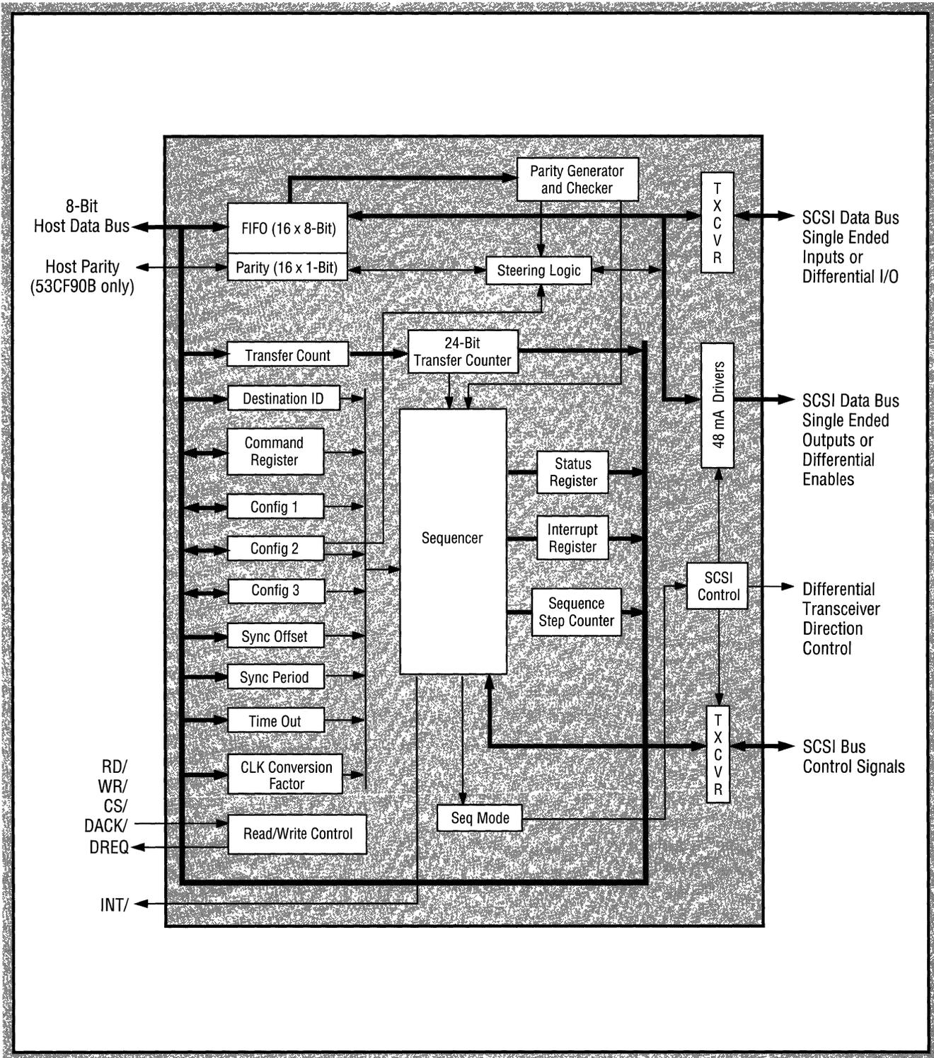
Figure 1-2. NCR 53CF90A, 53CF90B Functional Signal Grouping
