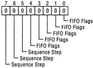
Synchronous Offset Register W (07h)
