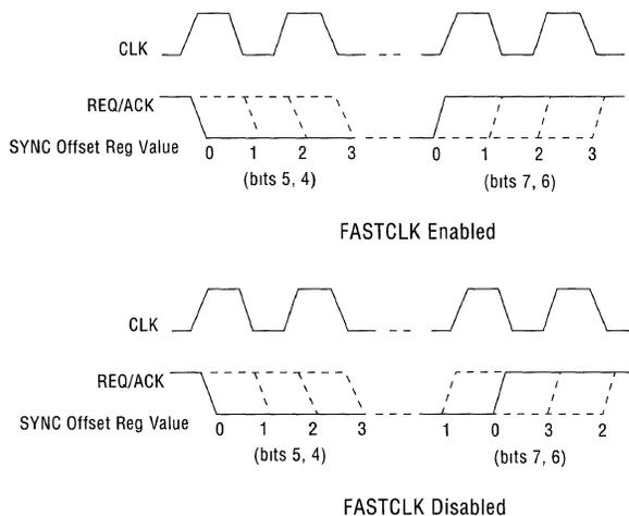
Note The input clock duty cycle affects the half clock assertion/deassertion delays
