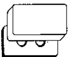
J2: Enable First Stage Zero-Wait State (Default: Pin 1 and 2 connected) (Pin 1 and 2 open)
