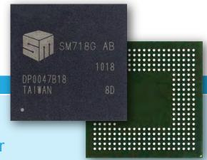
The SM718 is a PCI 2D multimedia mobile display controller device, packaged in a 320-pin BGA. Designed to complement needs for the embedded industry, it provides video and 2D capability. To help reduce system costs, it supports a wide variety of I/O, including analog RGB and digital LCD Panel interfaces, two Zoom Video interfaces, and Pulse Width Modulation (PWM). There are additional GPIO bits that can be used to interface to external devices as well.
