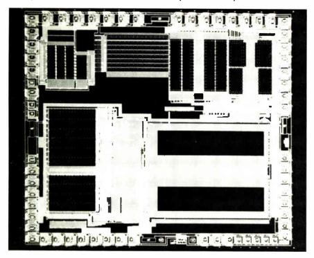
conjunction with one to four 7301 chips that provide an interface to a frame buffer up to 1 megabyte in size, the 7300 can unburden the host processor by taking over a variety of graphics-processing tasks. These include computation of picture-element addresses for the frame buffer, control of frame-buffer refreshing and timing, and handling direct-memoryaccess control.
