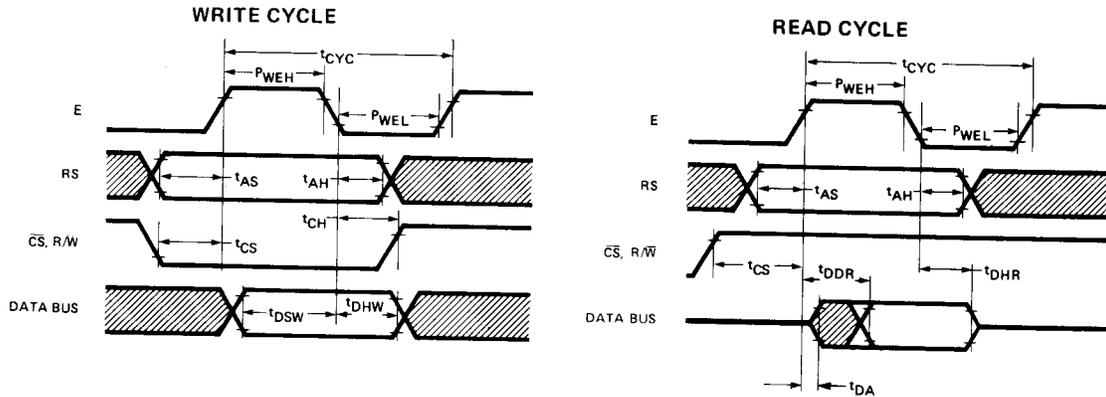
**Write Timing Characteristics** ( $V_{CC} = 5.0V \pm 5\%$ ,  $T_A = 0 - 70^\circ C$ , unless otherwise noted)
