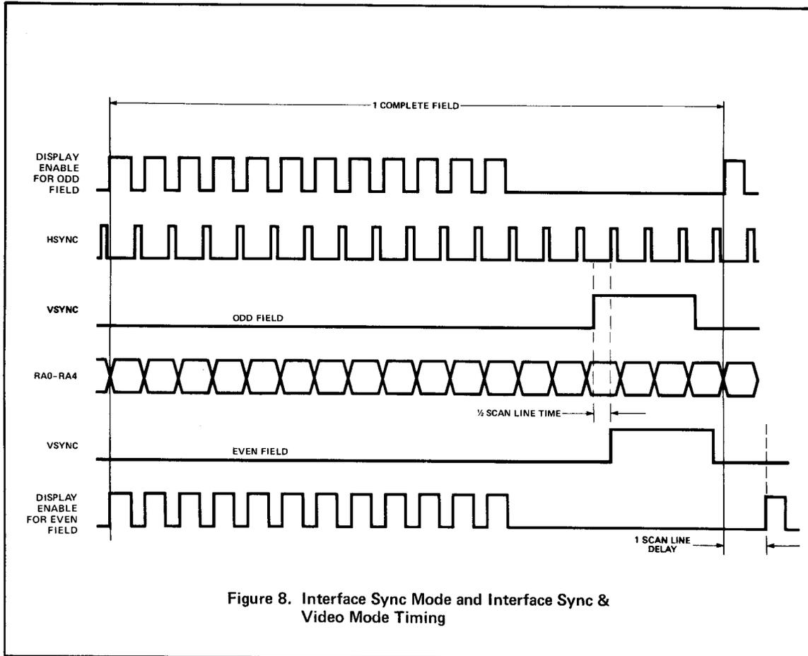
Figure 8. Interface Sync Mode and Interface Sync & Video Mode Timing
