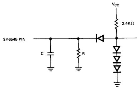
R = 11K $\Omega$  FOR DB<sub>0</sub>-DB<sub>7</sub>
