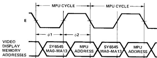
Figure 6.  $\phi 1/\phi 2$  Interleaving.
