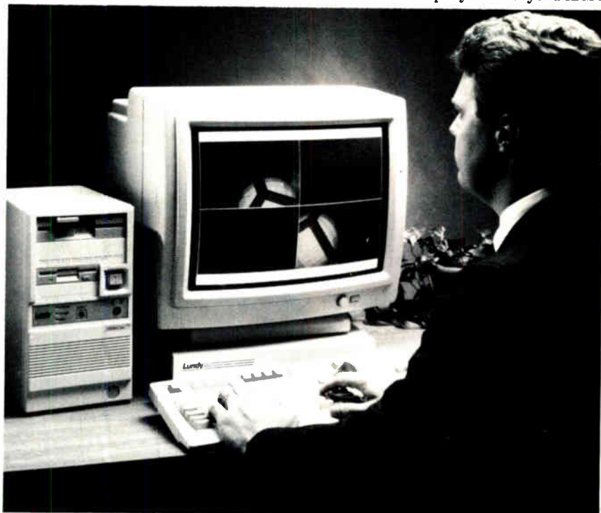
At the high end of the resolution scale is the Lundy 1612 Personal Graphics Workstation, which offers 1,600 by 1,200 pixels with 16 colors. It's based on the Texas Instruments 34010 processor.
