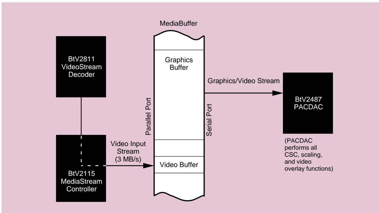
only the bandwidth necessary to fill the video buffer is consumed on the DRAM port of the MediaBuffer. For a CIF resolution video stream at 30 fps, this is only 4.6 MB/s. This results in approximately 95 MB/s of unused bandwidth available for other functions such as graphics and/or additional video windows.
