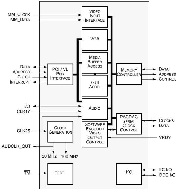
Figure 3. BtV2115 PCI-Bus Block Diagram
