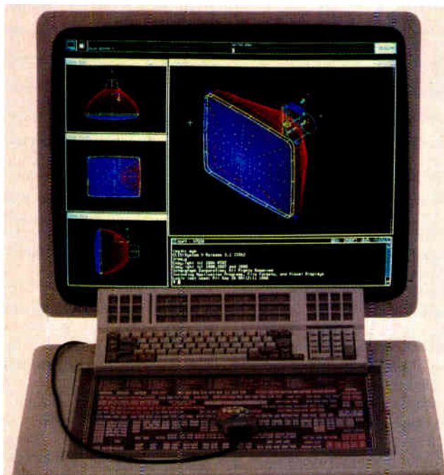
A screen measuring 27 in. on the diagonal, which displays 1,664 by 1,248 pixels, is available on Intergraph's model 3070 work station.
