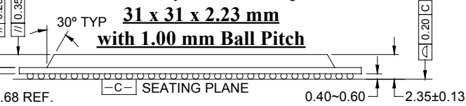
Figure 7. Mechanical Specifications - 681-Pin HSBGA Ball Grid Array Package with Heat Spreader
