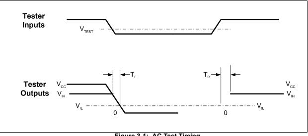
Figure 3-1: AC Test Timing
