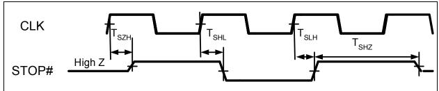
Figure 3-5: PCI Bus Stop Timing
