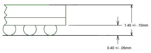
Figure 4-2: 256 Ball - Mini Ball Grid Array
