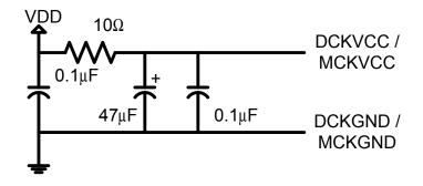
The suggested method for layout assumes a multilayer board including VCC and GND planes. All ground connections should be made as close to the pin/component as possible. The CVCC trace should route from the graphics controller through the pads of the filter components. The trace should NOT be connected to the filter components by a stub. All components (particularly the nearest  $0.1\mu$ F capacitor) should be placed as close as possible to the graphics controller.
