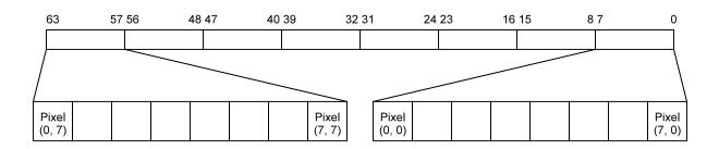
Figure E-9: Monochrome Pattern Data -- Occupies a Single Quadword
