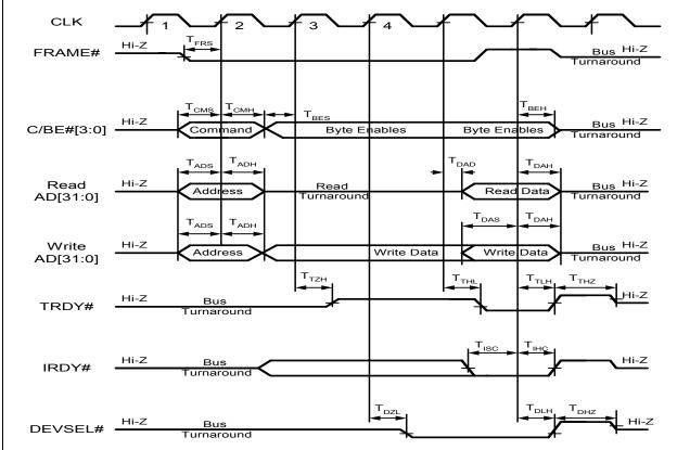
Figure 3-4: PCI Bus Frame Timing ractorictics DCI Rue Stop (CI K-22MU-)
