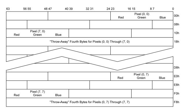
Figure E-12: 24bpp Pattern Data -- Occupies 256 Bytes (32 Quadwords)
