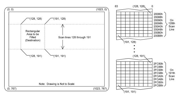
Figure E-13: On-Screen Destination for Example Pattern Fill BitBLT
