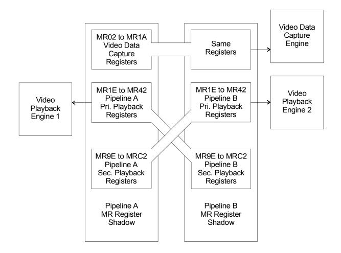
As shown, there is one set of registers for the video data capture engine, and this set is shared between both pipelines at register locations MR02-MR1A -- i.e., this one set of registers is accessible at register locations MR02-MR1A in both shadows of the MR register set.
