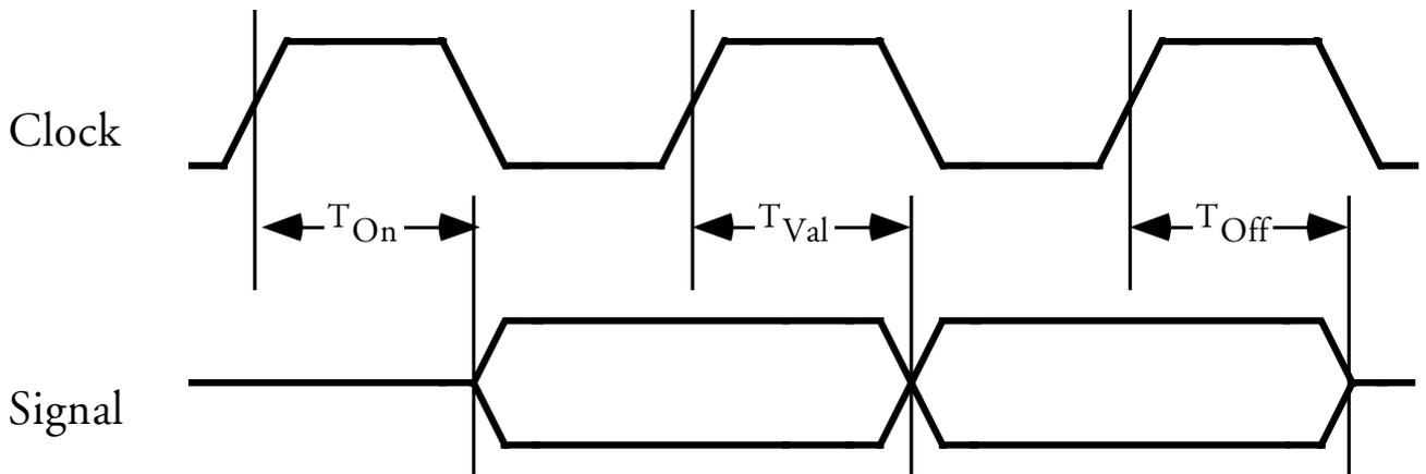
Figure 12.2 Output Timing Parameters
