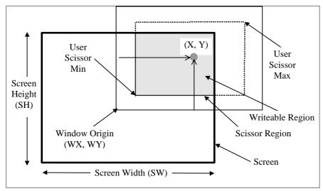
Figure 3-1 Screen Scissor and User Scissor Tests
