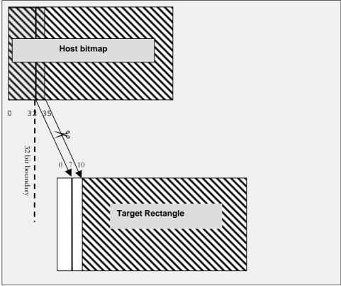
required, in this case we would rasterize the left edge to start at pixel 7. This aligns the source bitmap data with the mask data produced by the rasterizer. But, in order to protect the 3 pixels that we would otherwise overwrite, we use the scissor clip and set its bounds to be those of the original rectangle.
