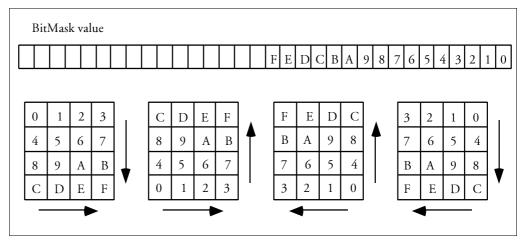
Figure 2-4 Relationship between Bitmask and Scanning Directions
