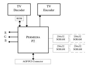
This reference board based on the Pervasive 3D solution, adds the necessary hardware to enable TV input and output.
