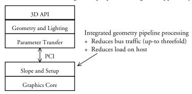
The geometry set-up unit accepts the coordinates of vertices plus color, depth, fog and texture parameters. It accepts the input parameters in either fixed point format or IEEE single precision floating point format; internal calculations are performed in floating point format. Vertex sharing for meshes, fans and polylines is supported with the shared vertices being loaded only once.
