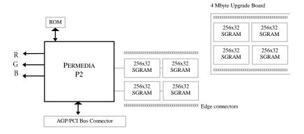
Designed for the business user or home enthusiast, this reference board adds extra memory for higher screen resolutions and extended local texture storage. This may be either a standard PCI board or an AGP card. As an AGP card, it would uses the DMA model to transfer textures into local memory where it caches them for higher performance.
