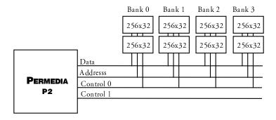
To minimize page breaks, PERMEDIA 2 can store and access data in memory as 2D patches. This is particularly useful for texture maps, where texture accesses can go in any direction through memory. By storing the data in a 2D format, the chances of a page break are reduced. 3Dlabs drivers allow configurable texture compression on download, saving memory and increasing performance.
