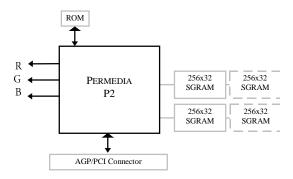
This board sets the standard for low-cost, high volume 3D, 2D and video acceleration. It is based on a PERMEDIA 2 with 2 Mbytes of memory and the option for an additional 2 Mbytes. It may be built as either a standard PCI board or as an AGP card. If an AGP card, it uses the AGP execute model to avoid storing textures locally; this frees memory for higher resolution screens.
