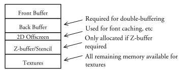
The multi-function nature of the memory organization allows PERMEDIA 2 to store the different buffers anywhere in the same physical memory, minimizing memory wastage and offering a simplified programming model. It is not necessary to store all data of a particular type together, so a texture map may be followed by a depth buffer or a framebuffer or another texture map.
