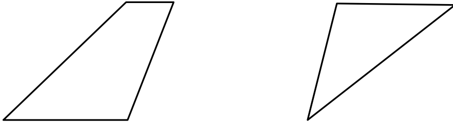
Figure 7.4 Screen aligned trapezoid and flat topped triangle
