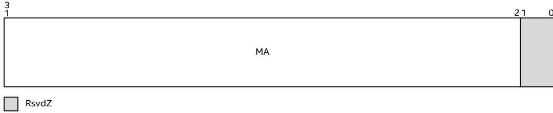
Figure 11-52. Performance Monitoring Interrupt Address Register
