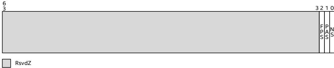
Figure 11-74. Virtual Command Capability Register
