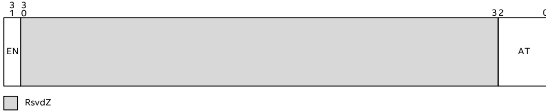
Figure 11-61. Performance Monitoring Address Type Filter Configuration Registers
