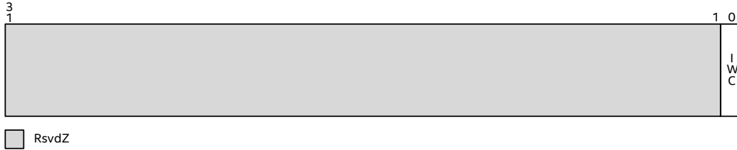
Figure 11-24. Invalidation Completion Status Register
