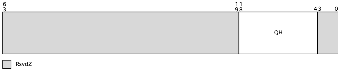
Figure 11-21. Invalidation Queue Head Register
