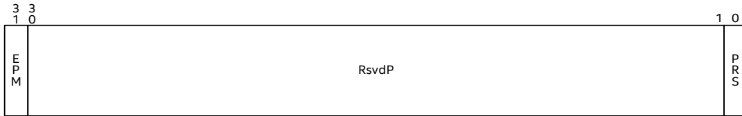
Figure 11-16. Protected Memory Enable Register
