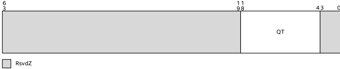
Figure 11-22. Invalidation Queue Tail Register
