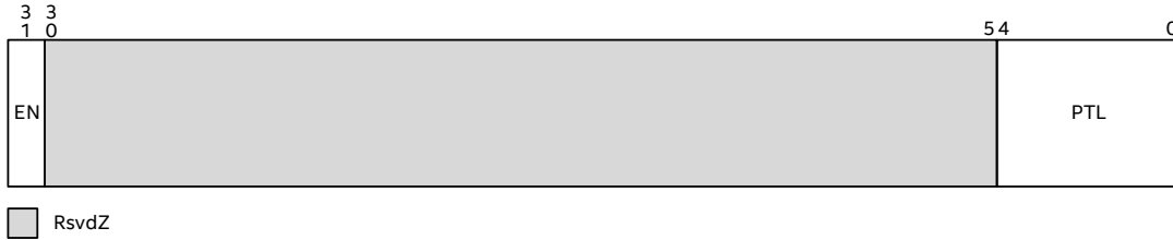
Figure 11-62. Performance Monitoring Page Table Level Filter Configuration Registers
