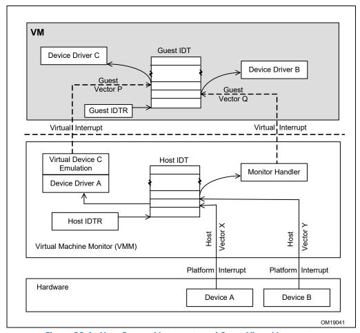
Figure 33-1. Host External Interrupts and Guest Virtual Interrupts
