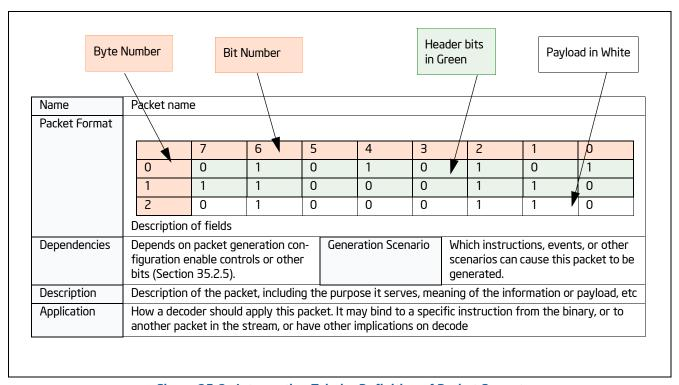
Figure 35-3. Interpreting Tabular Definition of Packet Format
