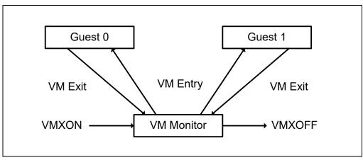
Figure 23-1. Interaction of a Virtual-Machine Monitor and Guests
