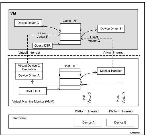
Figure 33-1. Host External Interrupts and Guest Virtual Interrupts
