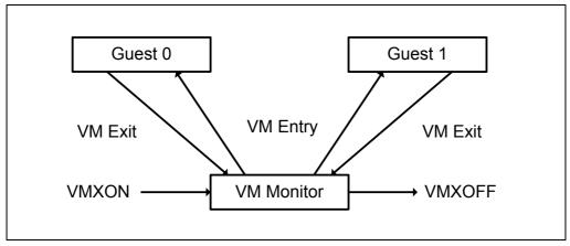
Figure 23-1. Interaction of a Virtual-Machine Monitor and Guests
