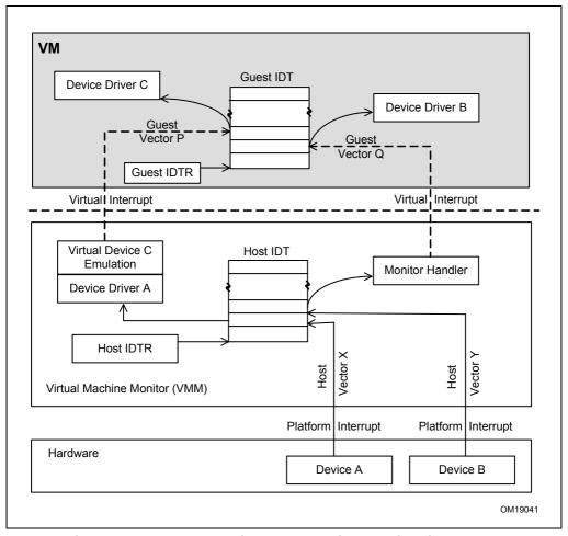
Figure 32-1. Host External Interrupts and Guest Virtual Interrupts
