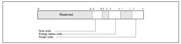
Figure 15-35. MSR\_RAPL\_POWER\_UNIT Register
