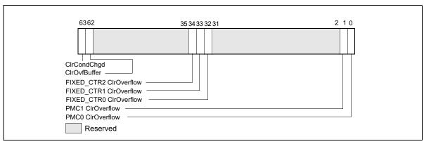
Figure 20-46. Layout of MSR\_PERF\_GLOBAL\_OVF\_CTRL MSR
