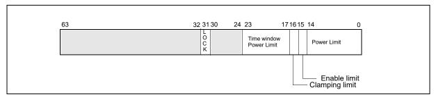
Figure 15-40. MSR\_PP0\_POWER\_LIMIT/MSR\_PP1\_POWER\_LIMIT Register
