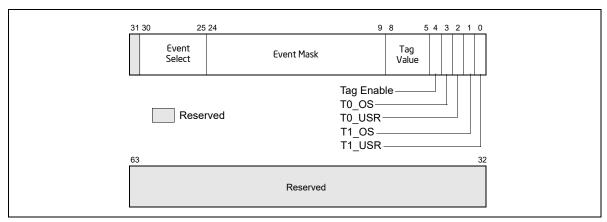
Figure 20-51. Event Selection Control Register (ESCR) for the Pentium 4 Processor, Intel® Xeon® Processor, and Intel® Xeon® Processor MP Supporting Hyper-Threading Technology
