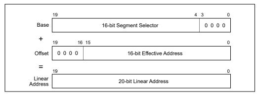
Figure 21-1. Real-Address Mode Address Translation
