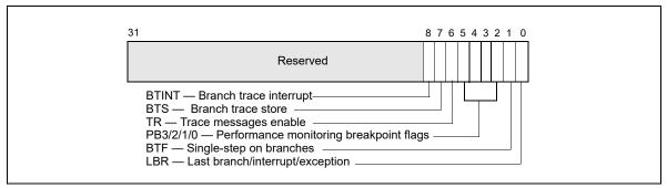
Figure 18-16. MSR DEBUGCTLB MSR for Pentium M Processors
