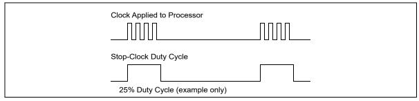
Figure 15-24. Processor Modulation Through Stop-Clock Mechanism
