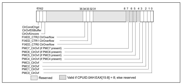
Figure 20-28. IA32\_PERF\_GLOBAL\_OVF\_CTRL MSR in Sandy Bridge Microarchitecture
