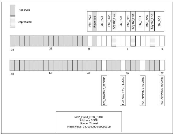
Figure 20-69. Layout of IA32\_FIXED\_CTR\_CTRL MSR Supporting Adaptive PEBS
