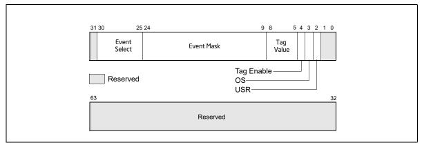
Figure 20-47. Event Selection Control Register (ESCR) for Pentium 4 and Intel® Xeon® Processors without Intel HT Technology Support
