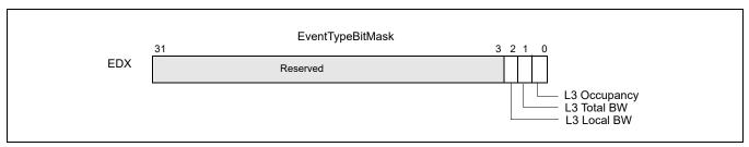
Figure 18-22. L3 Cache Monitoring Capability Enumeration Event Type Bit Vector (CPUID.(EAX=0FH, ECX=1H))
