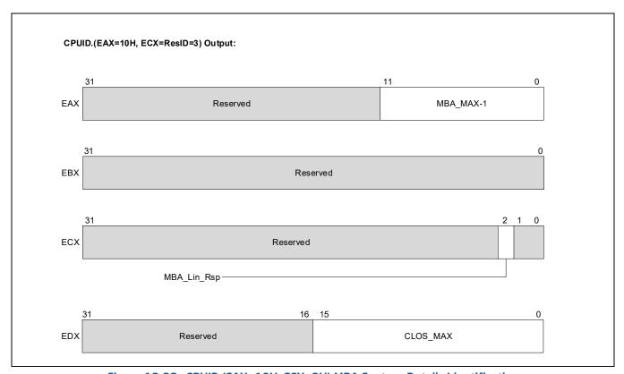
Figure 18-38. CPUID.(EAX=10H, ECX=3H) MBA Feature Details Identification
