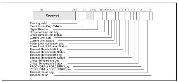
Figure 15-10. IA32\_THERM\_STATUS Register With HWP Feedback
