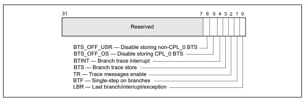
Figure 18-12. MSR DEBUGCTLA MSR for Pentium 4 and Intel Xeon Processors
