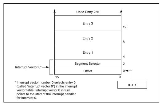
Figure 21-2. Interrupt Vector Table in Real-Address Mode
