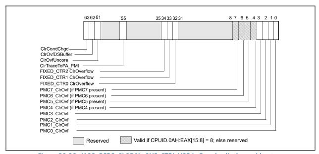
Figure 20-36. IA32\_PERF\_GLOBAL\_OVF\_CTRL MSR in Broadwell microarchitecture
