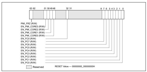
Figure 20-19. Layout of MSR\_UNCORE\_PERF\_GLOBAL\_CTRL MSR
