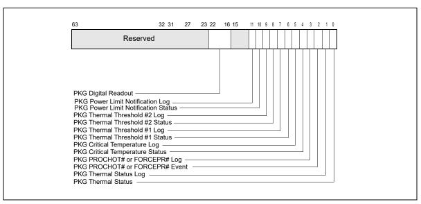
Figure 15-33. IA32\_PACKAGE\_THERM\_STATUS Register
