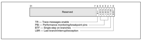
Figure 18-18. DEBUGCTLMSR Register (P6 Family Processors)
