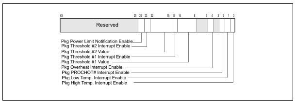
Figure 15-34. IA32\_PACKAGE\_THERM\_INTERRUPT Register
