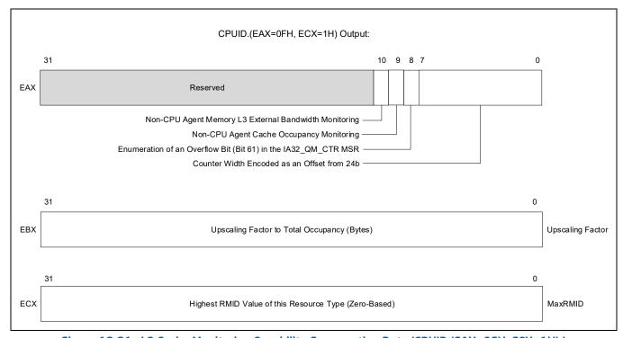
Figure 18-21. L3 Cache Monitoring Capability Enumeration Data (CPUID.(EAX=0FH, ECX=1H))
