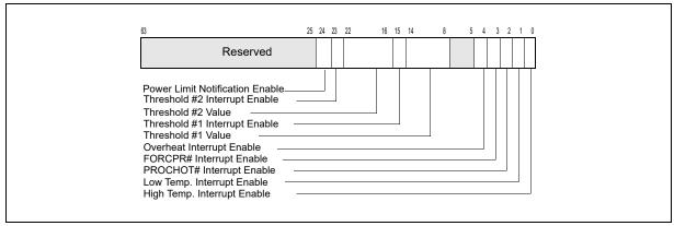
Figure 15-32. IA32\_THERM\_INTERRUPT Register
