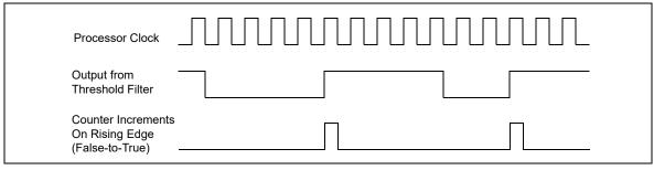
Figure 20-50. Effects of Edge Filtering
