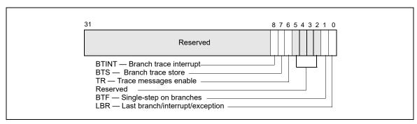
Figure 18-14. IA32\_DEBUGCTL MSR for Intel® Core™ Solo and Intel® Core™ Duo Processors
