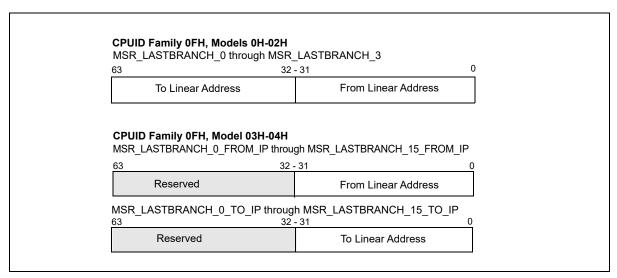
Figure 18-13. LBR MSR Branch Record Layout for the Pentium 4 and Intel® Xeon® Processor Family
