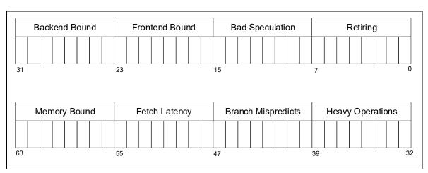
Figure 20-38. PERF\_METRICS MSR Definition for 12th Generation Intel® Core™ Processor P-core
