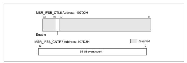
Figure 20-57. MSR IFSB CTL6, Address: 107D2H; MSR IFSB CNTR7, Address: 107D3H
