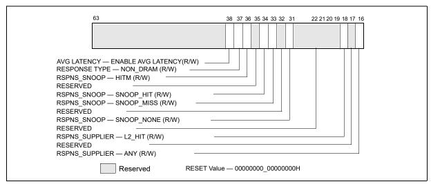
Figure 20-41. Response\_Supplier and Snoop Info Fields for MSR\_OFFCORE\_RSPx
