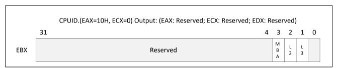
Figure 18-31. CPUID.(EAX=10H, ECX=0H) Available Resource Type Identification
