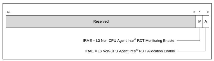
Figure 18-40. Layout of the IA32\_L3\_IO\_RDT\_CFG MSR for Enabling Non-CPU Agent Intel® RDT
