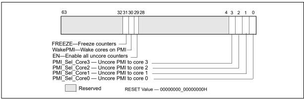
Figure 20-33. Layout of MSR UNC PERF GLOBAL CTRL MSR for Uncore
