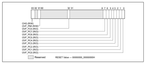
Figure 20-20. Layout of MSR\_UNCORE\_PERF\_GLOBAL\_STATUS MSR
