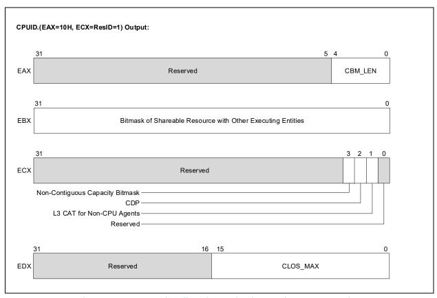
Figure 18-32. L3 Cache Allocation Technology and CDP Enumeration
