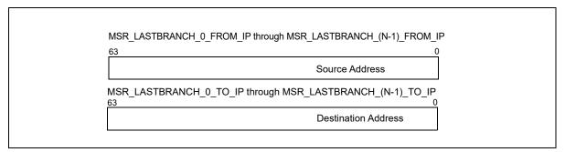
Figure 18-4. 64-bit Address Layout of LBR MSR
