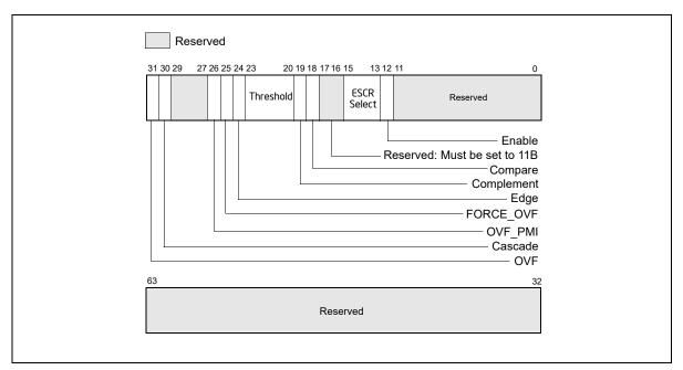
Figure 20-49. Counter Configuration Control Register (CCCR)
