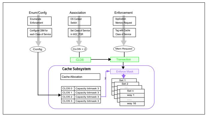
Figure 18-28. Class of Service and Cache Capacity Bitmasks
