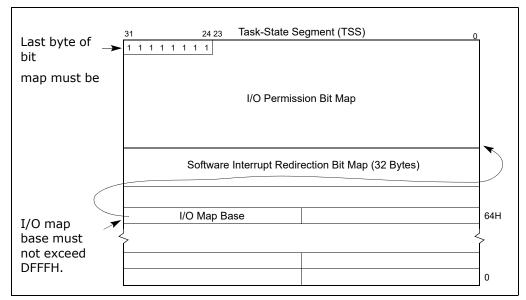
Figure 21-5. Software Interrupt Redirection Bit Map in TSS
