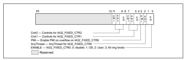
Figure 20-7. IA32\_FIXED\_CTR\_CTRL MSR Supporting Architectural Performance Monitoring Version 3
