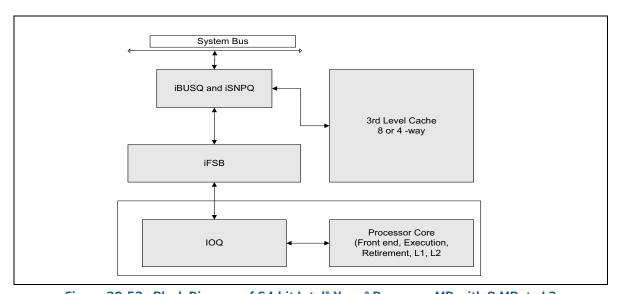
Figure 20-53. Block Diagram of 64-bit Intel® Xeon® Processor MP with 8-MByte L3
