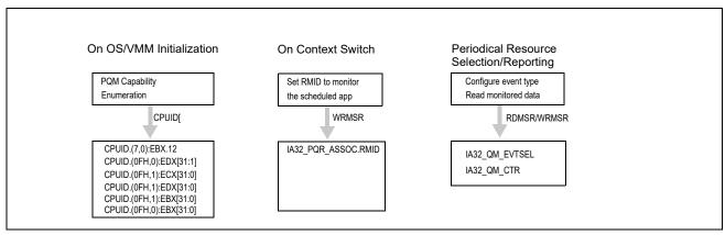
Figure 18-19. Platform Shared Resource Monitoring Usage Flow
