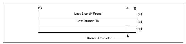
Figure 18-9. 64-bit Branch Trace Record Format
