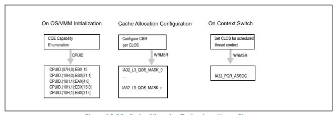
Figure 18-30. Cache Allocation Technology Usage Flow
