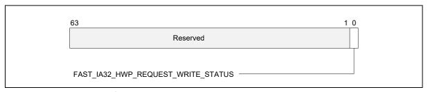
Figure 15-15. FAST\_UNCORE\_MSRS\_STATUS MSR
