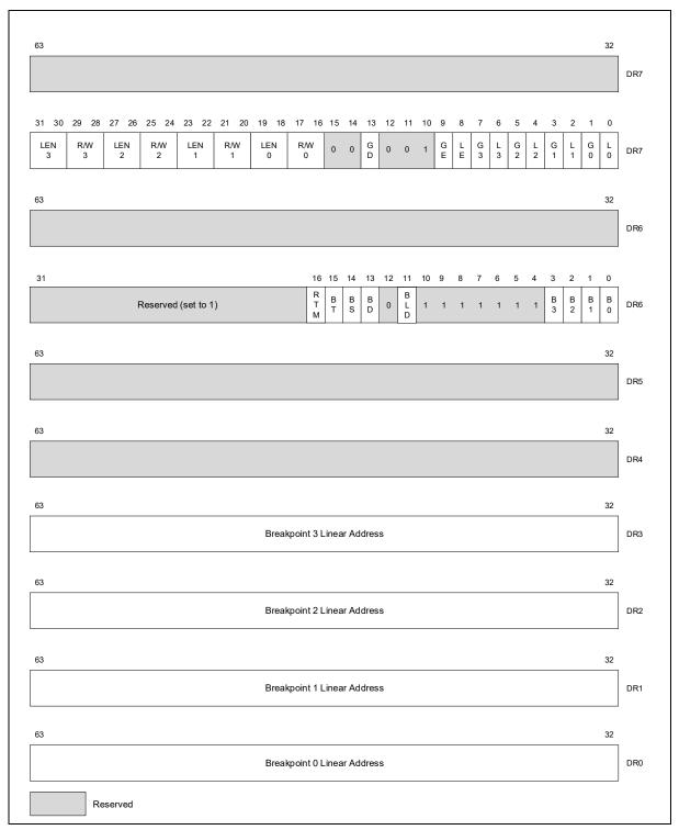
Figure 18-2. DR6/DR7 Layout on Processors Supporting Intel® 64 Architecture
