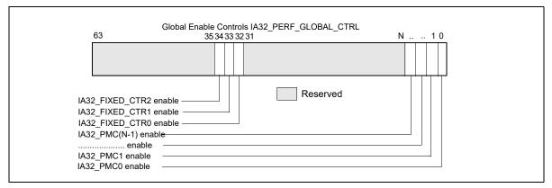
Figure 20-8. Layout of Global Performance Monitoring Control MSR
