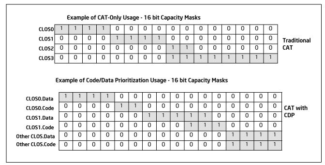
Figure 18-29. Code and Data Capacity Bitmasks of CDP
