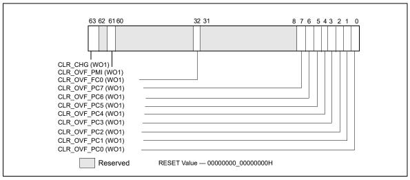
Figure 20-21. Layout of MSR UNCORE PERF GLOBAL OVF CTRL MSR
