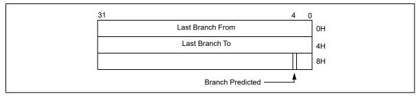
Figure 18-6. 32-bit Branch Trace Record Format
