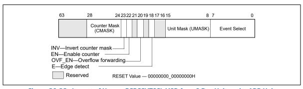
Figure 20-32. Layout of Uncore PERFEVTSEL MSR for a C-Box Unit or the ARB Unit
