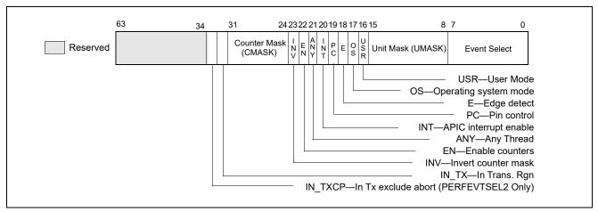
Figure 20-34. Layout of IA32\_PERFEVTSELx MSRs Supporting Intel TSX
