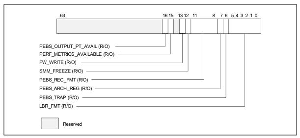
Figure 20-65. Layout of IA32\_PERF\_CAPABILITIES MSR
