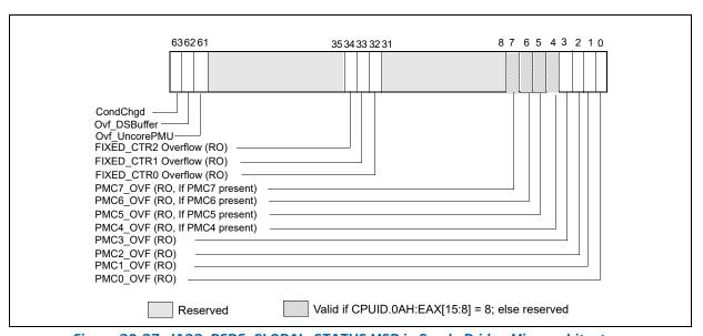
Figure 20-27. IA32\_PERF\_GLOBAL\_STATUS MSR in Sandy Bridge Microarchitecture
