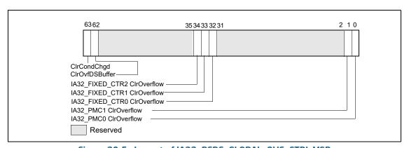
Figure 20-5. Layout of IA32\_PERF\_GLOBAL\_OVF\_CTRL MSR
