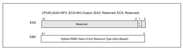
Figure 18-20. CPUID.(EAX=0FH, ECX=0H) Monitoring Resource Type Enumeration
