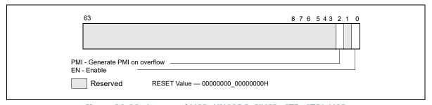
Figure 20-23. Layout of MSR\_UNCORE\_FIXED\_CTR\_CTRL MSR
