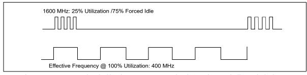
Figure 15-23. Example of Effective Frequency Reduction and Forced Idle Period of HDC
