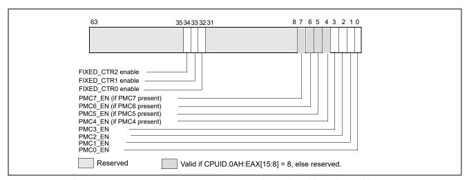
Figure 20-26. IA32\_PERF\_GLOBAL\_CTRL MSR in Sandy Bridge Microarchitecture
