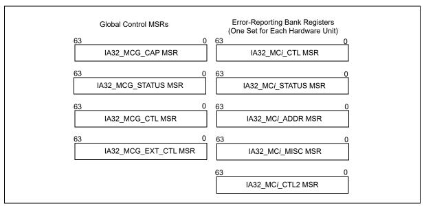
Figure 16-1. Machine-Check MSRs
