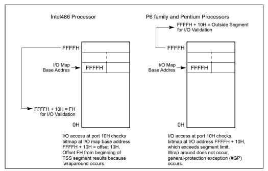
Figure 23-1. I/O Map Base Address Differences
