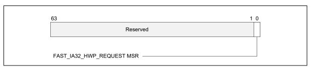
Figure 15-13. FAST UNCORE MSRS CAPABILITY MSR
