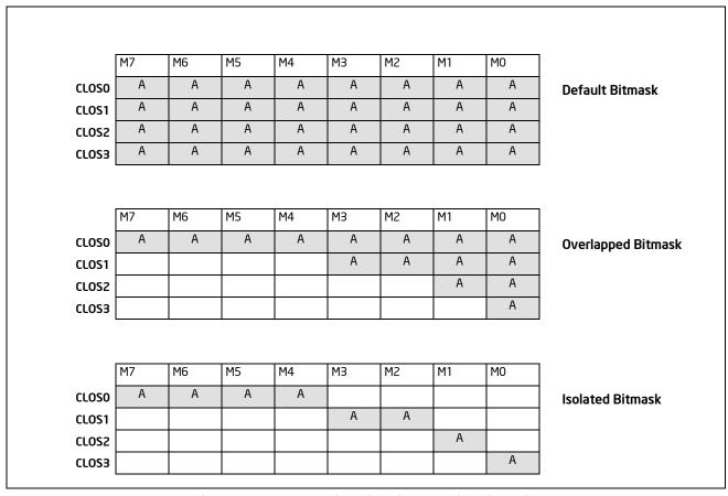
Figure 18-27. Examples of Cache Capacity Bitmasks
