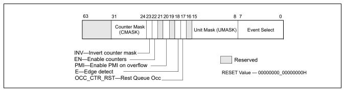
Figure 20-22. Layout of MSR\_UNCORE\_PERFEVTSELx MSRs
