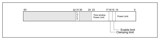
Figure 15-44. MSR\_DRAM\_POWER\_LIMIT Register
