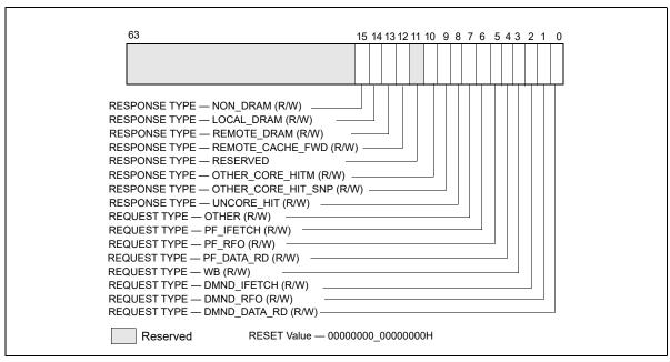
Figure 20-18. Layout of MSR\_OFFCORE\_RSP\_0 and MSR\_OFFCORE\_RSP\_1 to Configure Off-core Response Events
