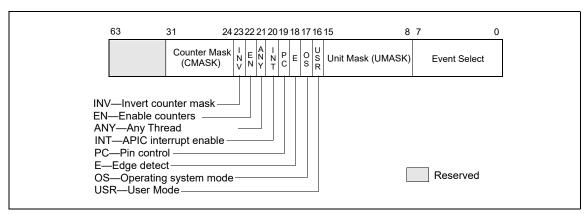
Figure 20-6. Layout of IA32\_PERFEVTSELx MSRs Supporting Architectural Performance Monitoring Version 3
