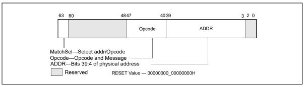
Figure 20-24. Layout of MSR\_UNCORE\_ADDR\_OPCODE\_MATCH MSR
