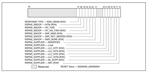
Figure 20-31. Response\_Supplier and Snoop Info Fields for MSR\_OFFCORE\_RSP\_x
