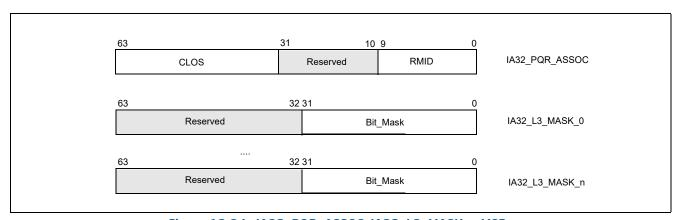
Figure 18-34. IA32\_PQR\_ASSOC, IA32\_L3\_MASK\_n MSRs
