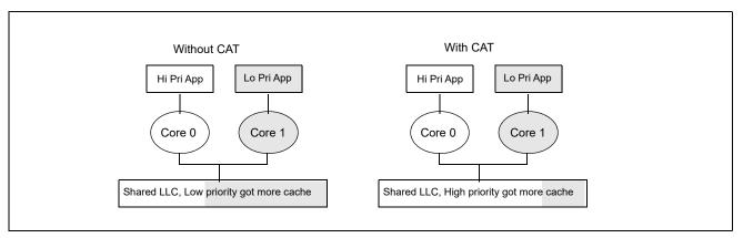
Figure 18-26. Cache Allocation Technology Enables Allocation of More Resources to High Priority Applications
