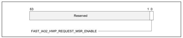
Figure 15-14. FAST\_UNCORE\_MSRS\_CTL MSR
