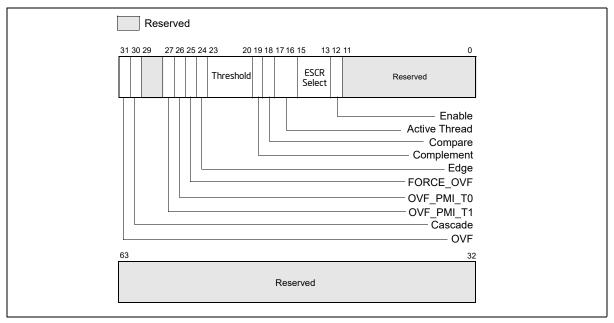
Figure 20-52. Counter Configuration Control Register (CCCR)
