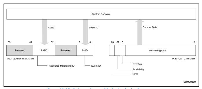
Figure 18-25. Software Usage of Cache Monitoring Resources
