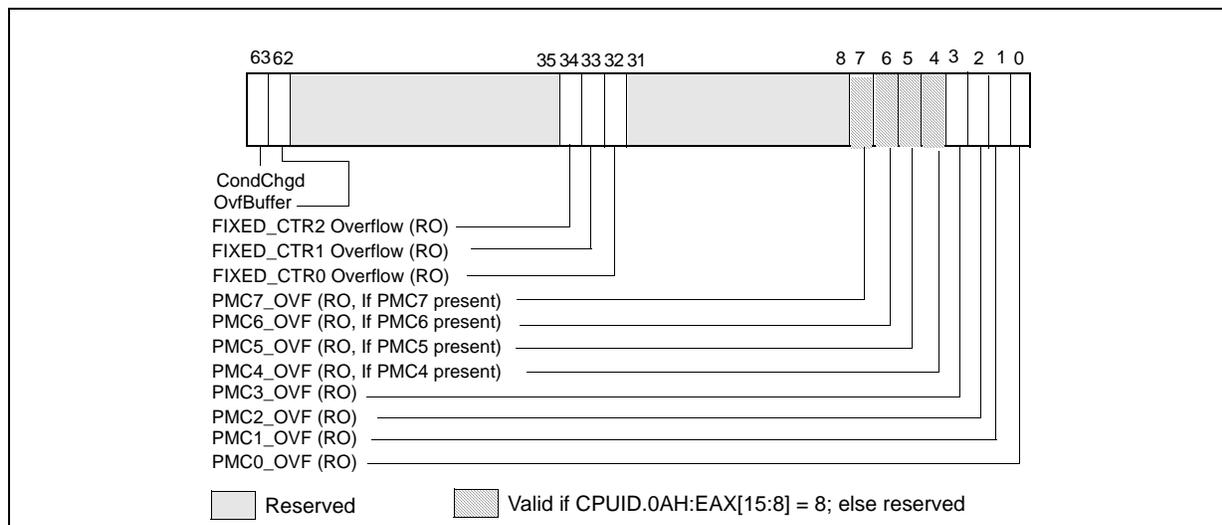
**Figure 18-27. IA32\_PERF\_GLOBAL\_STATUS MSR in Intel® Microarchitecture Code Name Sandy Bridge**
