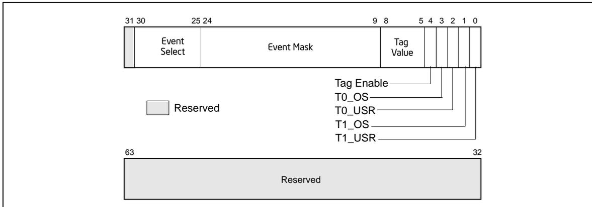
**Figure 18-39. Event Selection Control Register (ESCR) for the Pentium 4 Processor, Intel Xeon Processor and Intel Xeon Processor MP Supporting Hyper-Threading Technology**
