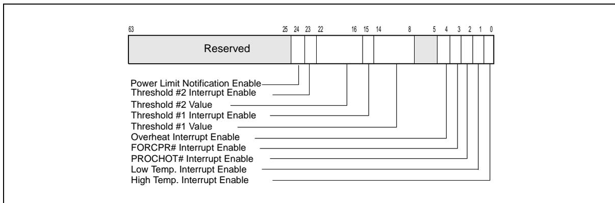
Figure 14-13. IA32\_THERM\_INTERRUPT Register
