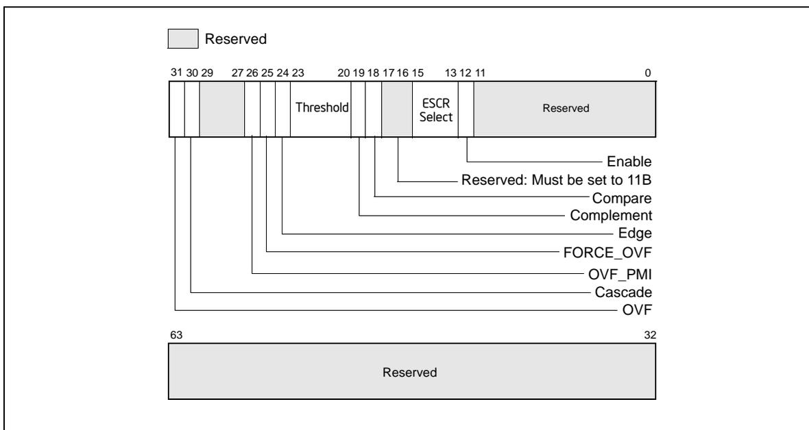
**Figure 18-37. Counter Configuration Control Register (CCCR)**
