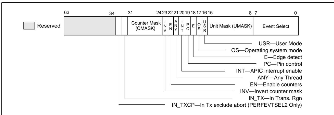
Figure 18-34. Layout of IA32\_PERFEVTSELx MSRs Supporting Intel TSX
