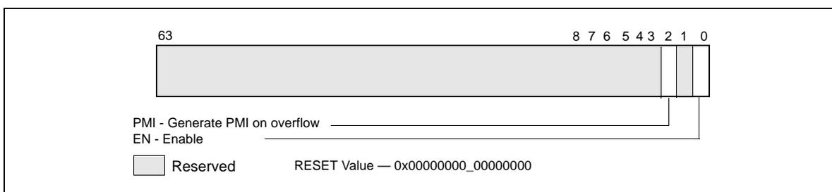
Figure 18-23. Layout of MSR\_UNCORE\_FIXED\_CTR\_CTRL MSR
