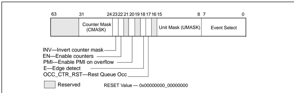
Figure 18-22. Layout of MSR\_UNCORE\_PERFEVTSELx MSRs
