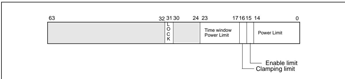
Figure 14-25. MSR\_DRAM\_POWER\_LIMIT Register
