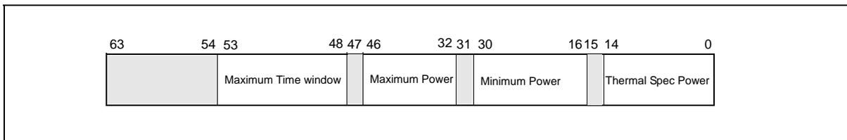
Figure 14-19. MSR\_PKG\_POWER\_INFO Register
