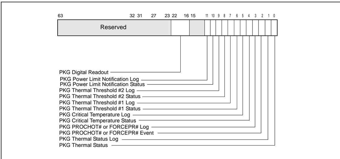
Figure 14-14. IA32\_PACKAGE\_THERM\_STATUS Register
