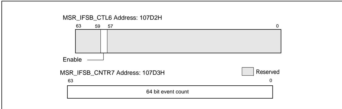
**Figure 18-46. MSR\_IFSB\_CTL6, Address: 107D2H;
