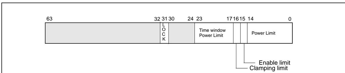
Figure 14-21. MSR\_PP0\_POWER\_LIMIT/MSR\_PP1\_POWER\_LIMIT Register
