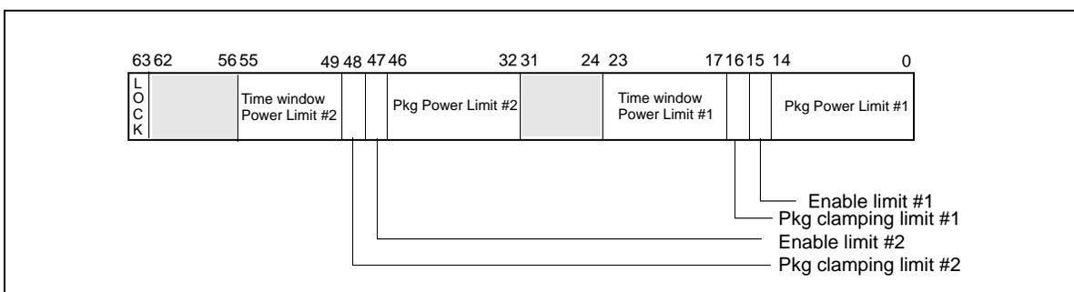
**Figure 14-17. MSR\_PKG\_POWER\_LIMIT Register**
