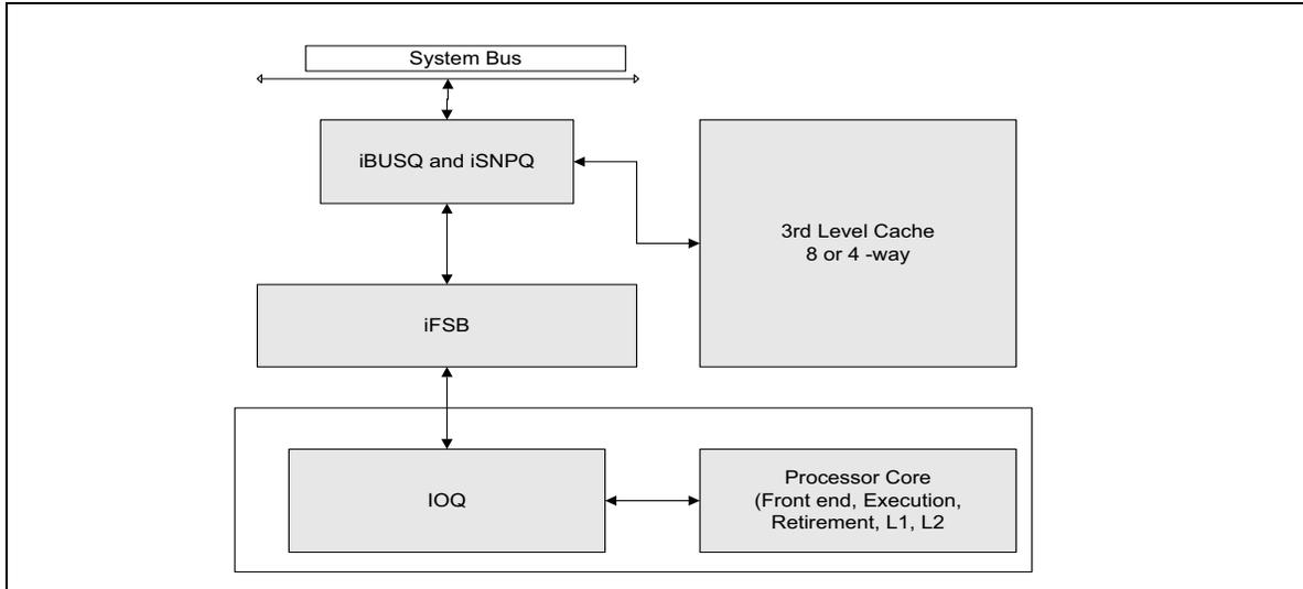
Figure 18-42. Block Diagram of 64-bit Intel Xeon Processor MP with 8-MByte L3
