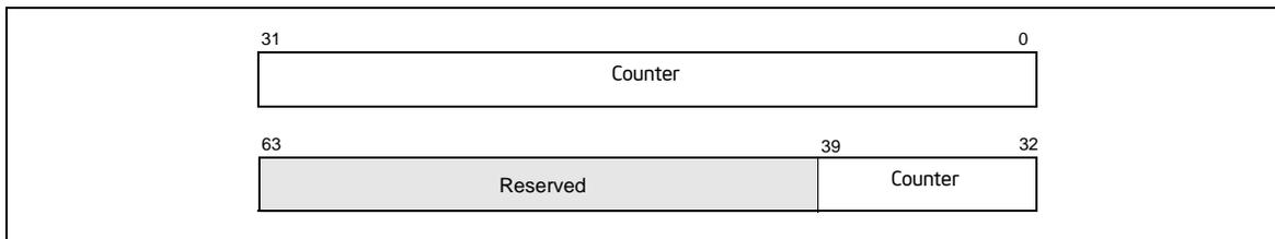
Figure 18-36. Performance Counter (Pentium 4 and Intel Xeon Processors)
