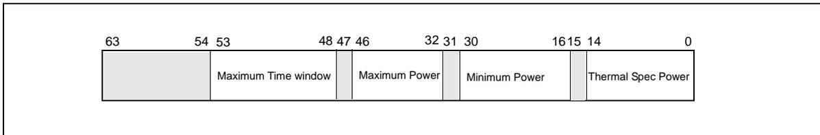
Figure 14-27. MSR\_DRAM\_POWER\_INFO Register
