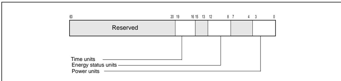
Figure 14-16. MSR\_RAPL\_POWER\_UNIT Register
