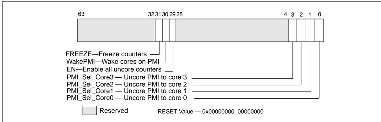
Figure 18-33. Layout of MSR\_UNC\_PERF\_GLOBAL\_CTRL MSR for Uncore
