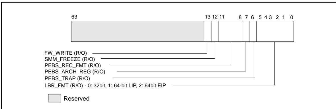
Figure 18-41. Layout of IA32\_PERF\_CAPABILITIES MSR
