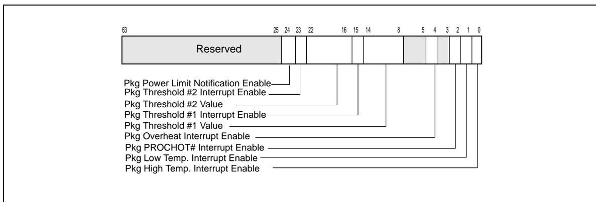
Figure 14-15. IA32\_PACKAGE\_THERM\_INTERRUPT Register
