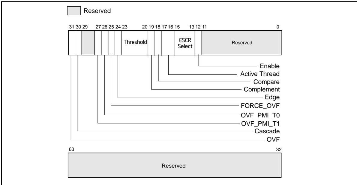
**Figure 18-40. Counter Configuration Control Register (CCCR)**
