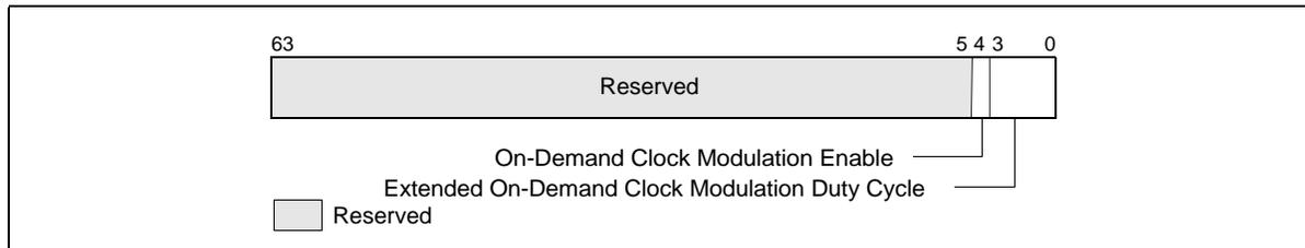
Figure 14-11. IA32\_CLOCK\_MODULATION MSR with Clock Modulation Extension
