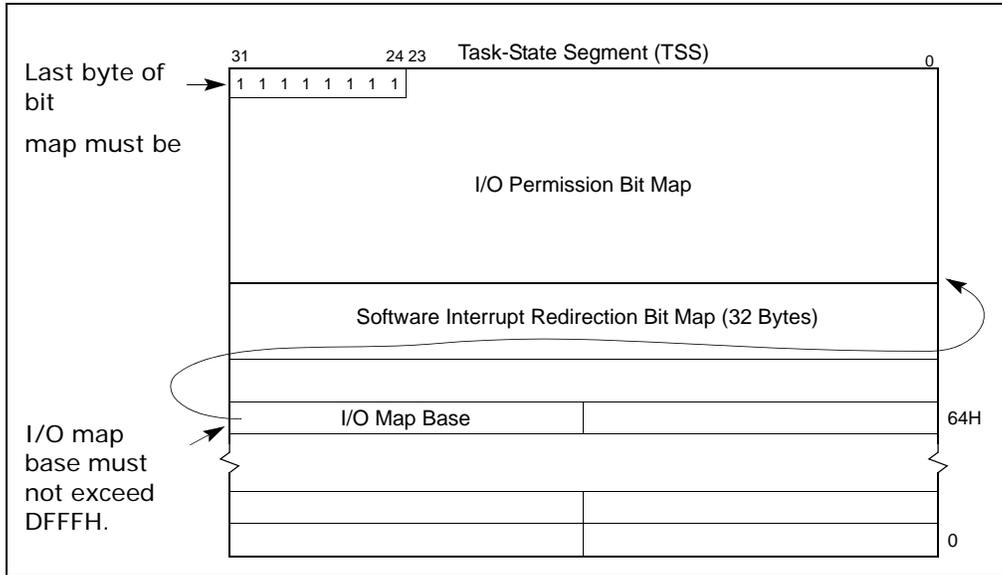
Figure 20-5. Software Interrupt Redirection Bit Map in TSS
