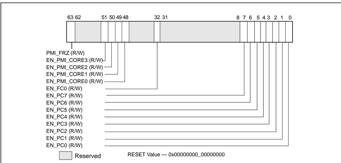
Figure 18-19. Layout of MSR\_UNCORE\_PERF\_GLOBAL\_CTRL MSR
