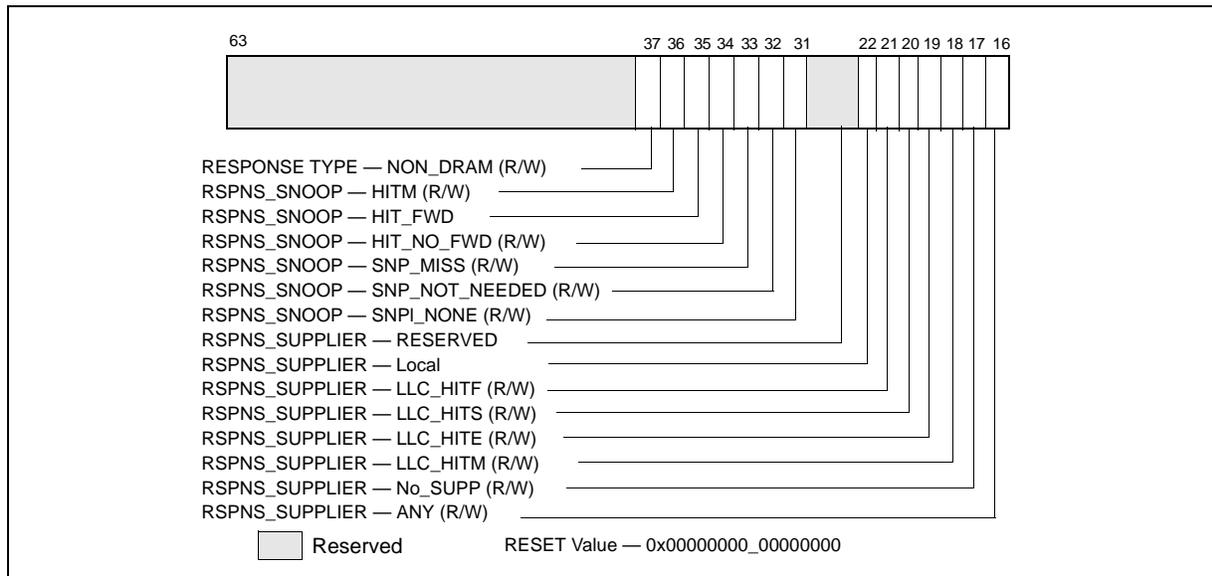
**Figure 18-31. Response\_Supplier and Snoop Info Fields for MSR\_OFFCORE\_RSP\_x**
