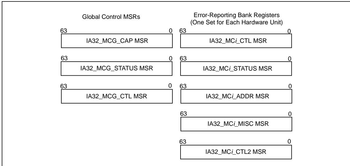
Figure 15-1. Machine-Check MSRs
