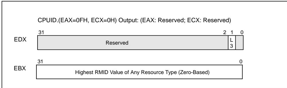
**Figure 17-19. CPUID.(EAX=0FH, ECX=0H) QoS Resource Type Enumeration**
