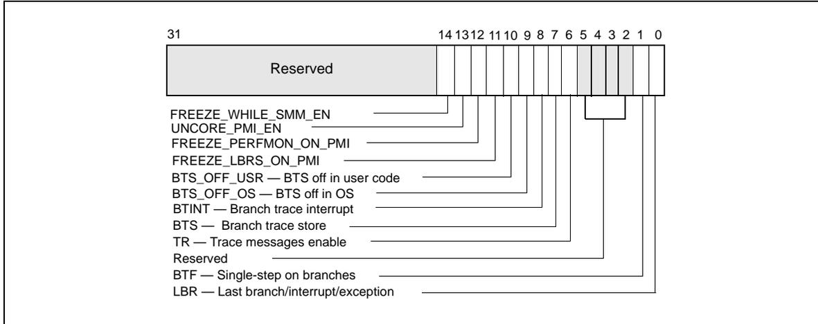
**Figure 17-11. IA32\_DEBUGCTL MSR for Processors based on Intel microarchitecture code name Nehalem**
