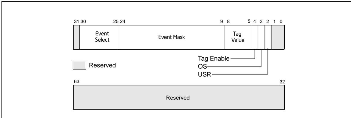
**Figure 18-35. Event Selection Control Register (ESCR) for Pentium 4 and Intel Xeon Processors without Intel HT Technology Support**
