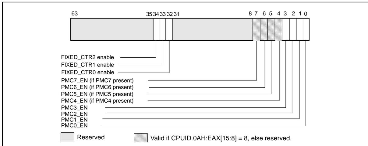
**Figure 18-26. IA32\_PERF\_GLOBAL\_CTRL MSR in Intel® Microarchitecture Code Name Sandy Bridge**
