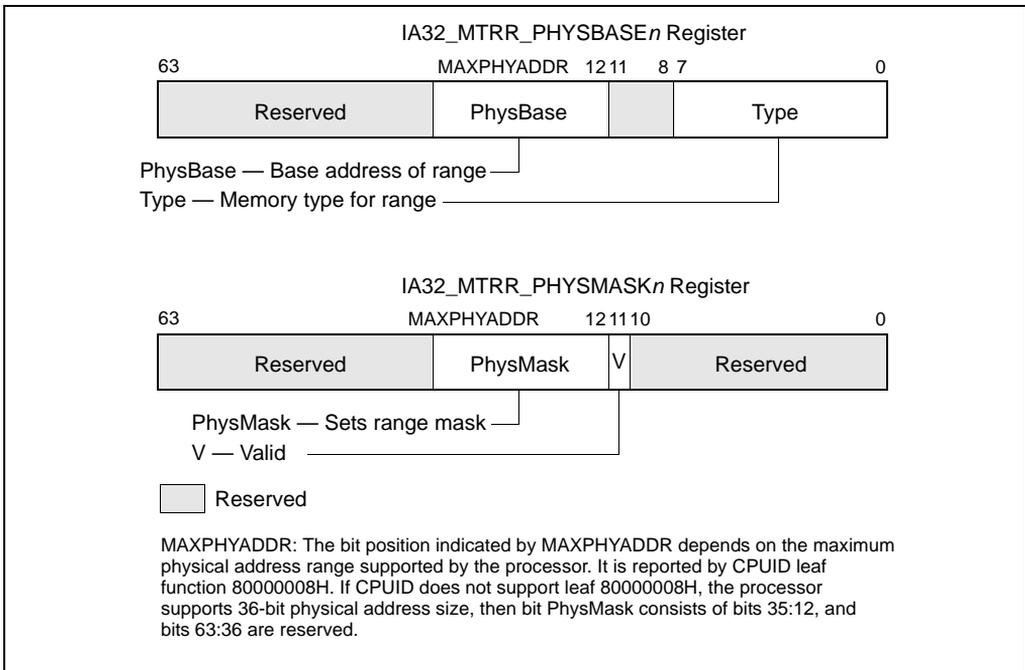
**Figure 10-6. IA32\_MTRR\_PHYSBASE<sub>n</sub> and IA32\_MTRR\_PHYSMASK<sub>n</sub> Variable-Range Register Pair**
