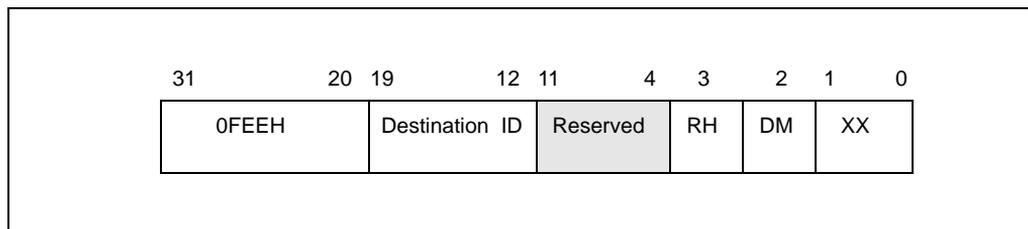
**Figure 8-24. Layout of the MSI Message Address Register**
