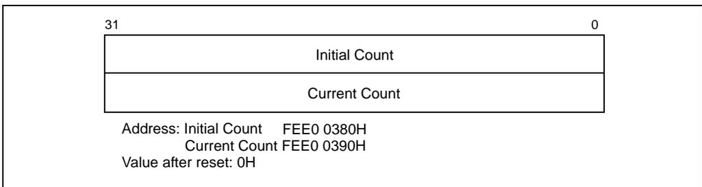
**Figure 8-11. Initial Count and Current Count Registers**
