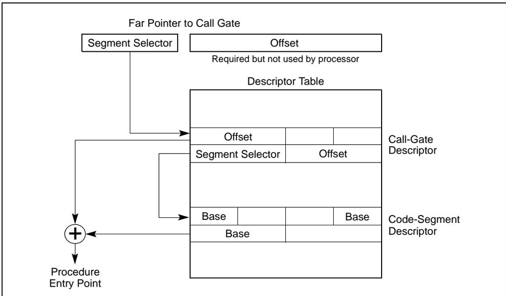
Figure 4-10. Call-Gate Mechanism
