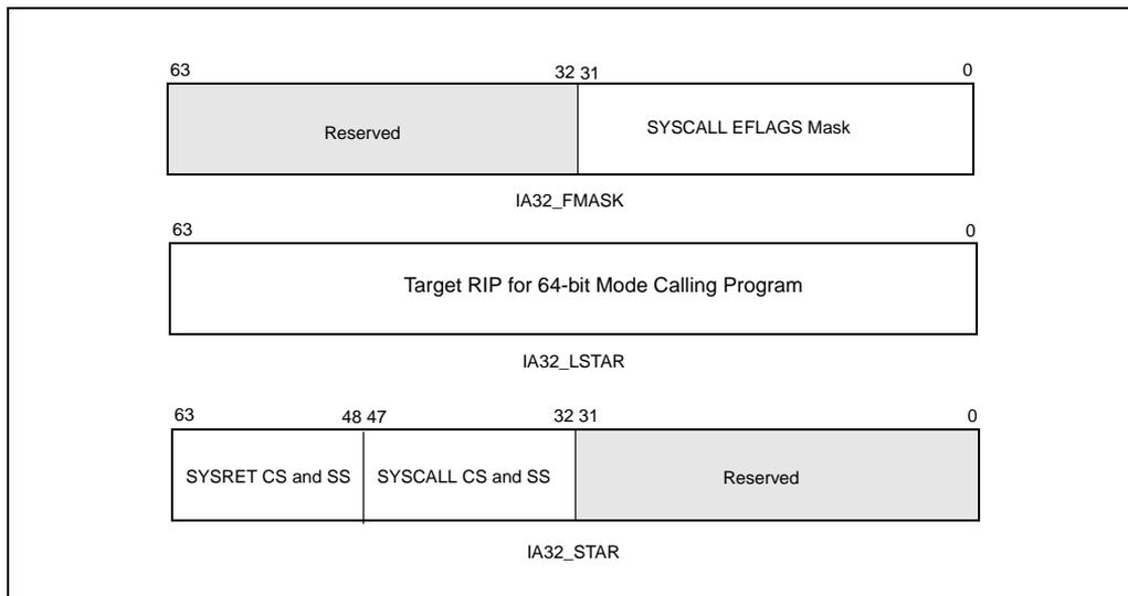
**Figure 4-14. MSRs Used by SYSCALL and SYSRET**
