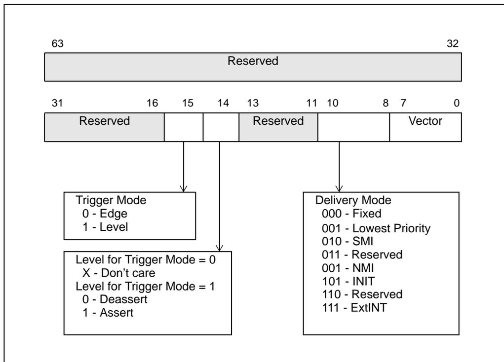
**Figure 8-25. Layout of the MSI Message Data Register**
