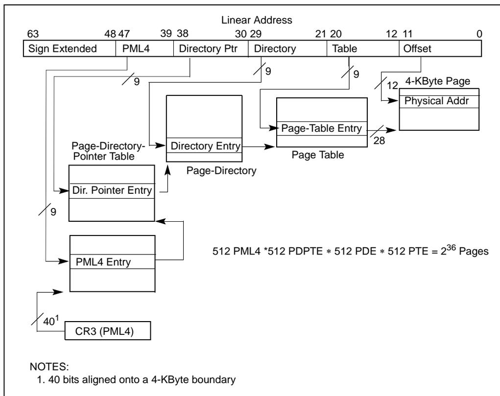
Figure 3-24. IA-32e Mode Paging Structures (4-KByte Pages)
