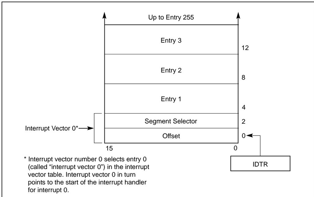
**Figure 15-2. Interrupt Vector Table in Real-Address Mode**
