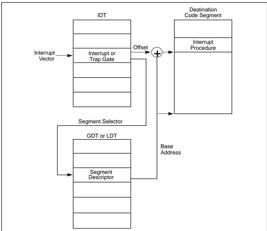
Figure 5-3. Interrupt Procedure Call
