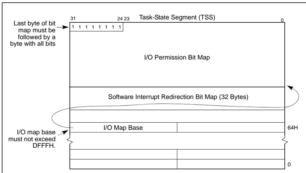
**Figure 15-5. Software Interrupt Redirection Bit Map in TSS**
