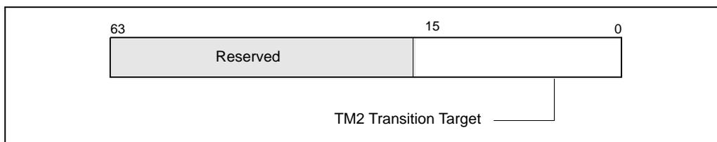
**Figure 13-4. MSR\_THERM2\_CTL Register for Supporting TM2**
