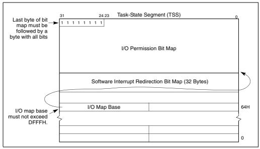
Figure 16-5. Software Interrupt Redirection Bit Map in TSS
