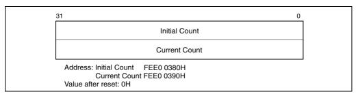
Figure 8-11. Initial Count and Current Count Registers
