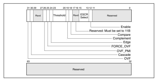
Figure 15-9. Counter Configuration Control Register (CCCR)
