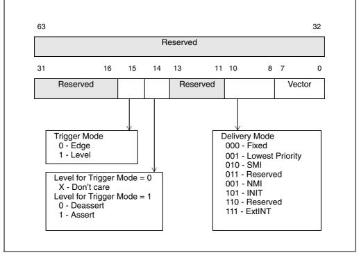
Figure 8-24. Layout of the MSI Message Data Register
