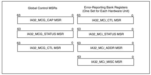
Figure 14-1. Machine-Check MSRs
