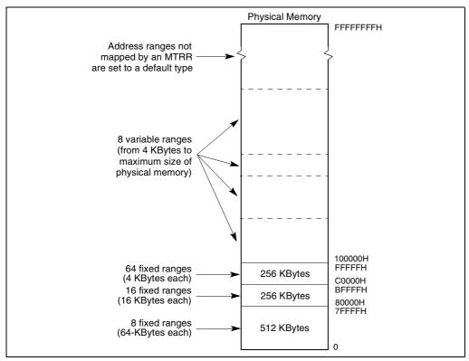
Figure 10-3. Mapping Physical Memory With MTRRs
