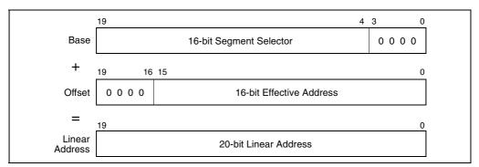
Figure 16-1. Real-Address Mode Address Translation
