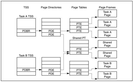
Figure 6-8. Overlapping Linear-to-Physical Mappings
