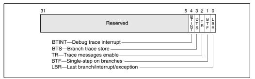
Figure 15-4. IA32\_DEBUGCTL MSR (Pentium 4 and Intel Xeon Processors)
