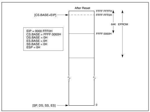
Figure 9-3. Processor State After Reset
