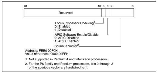
Figure 8-22. Spurious-Interrupt Vector Register (SVR)
