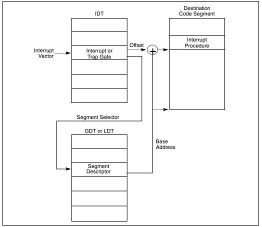
Figure 5-3. Interrupt Procedure Call
