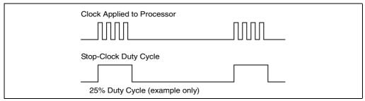
Figure 13-6. Processor Modulation Through Stop-Clock Mechanism
