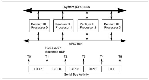
Figure C-1. MP System With Multiple Pentium III Processors
