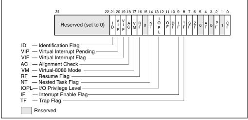
Figure 2-3. System Flags in the EFLAGS Register
