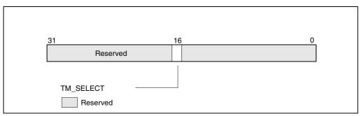
Figure 13-7. MSR\_THERM2\_CTL Register for the Pentium M Processor
