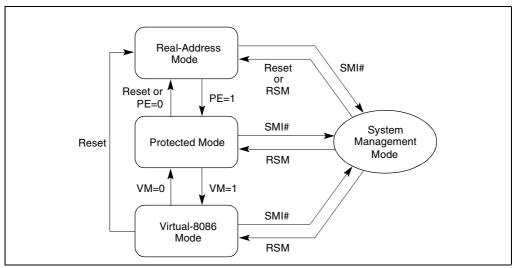
Figure 2-2 shows how the processor moves among these operating modes.
