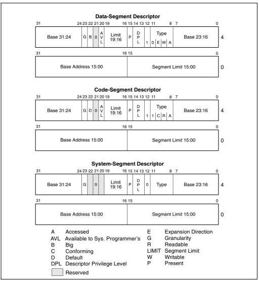
Figure 4-1. Descriptor Fields Used for Protection
