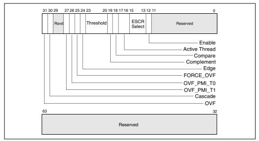
Figure 15-16. Counter Configuration Control Register (CCCR)
