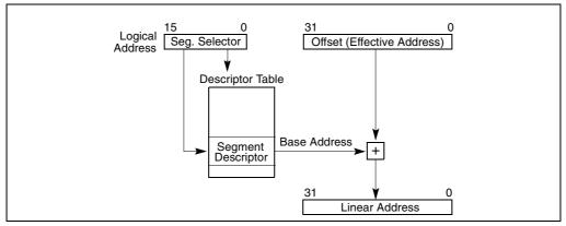
Figure 3-5. Logical Address to Linear Address Translation
