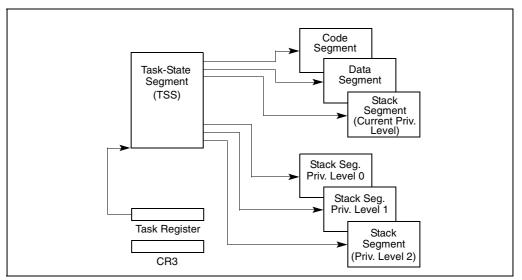
Figure 6-1. Structure of a Task
