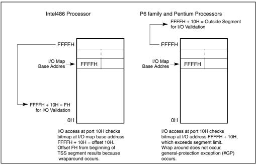
Figure 18-1. I/O Map Base Address Differences
