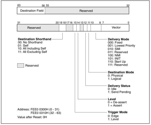
Figure 8-12. Interrupt Command Register (ICR)
