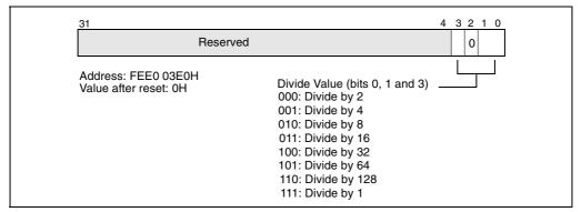
Figure 8-10. Divide Configuration Register
