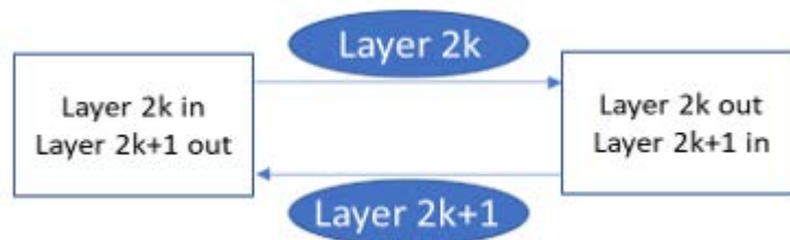
Figure 20-13. Minimal Memory Footprint Buffer Allocation Scheme for Trivial Deep Learning Topology
