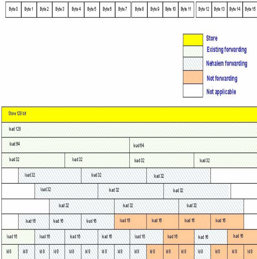
Figure 4-3. Store-Forwarding Scenarios of 16-Byte Store Operations
