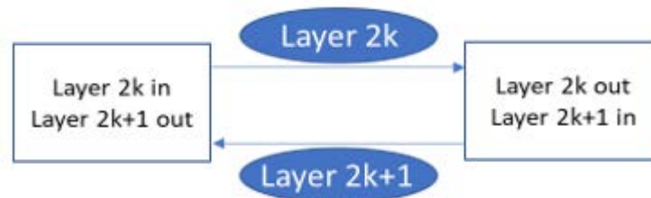
Figure 20-15. Minimal Memory Footprint Buffer Allocation Scheme for the Trivial Deep Learning Topology
