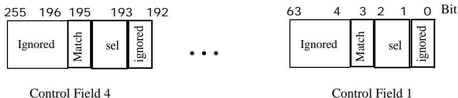
Figure 5-20. VPERMIL2PD Control Field
