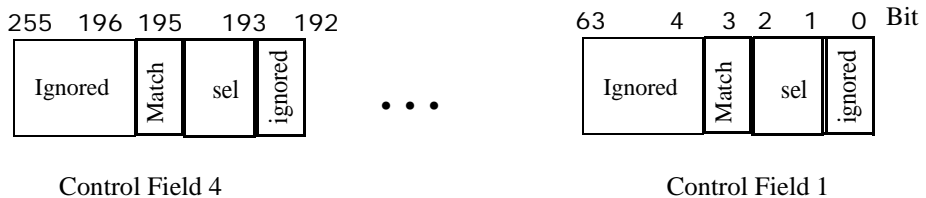
Figure 5-20. VPERMIL2PD Control Field
