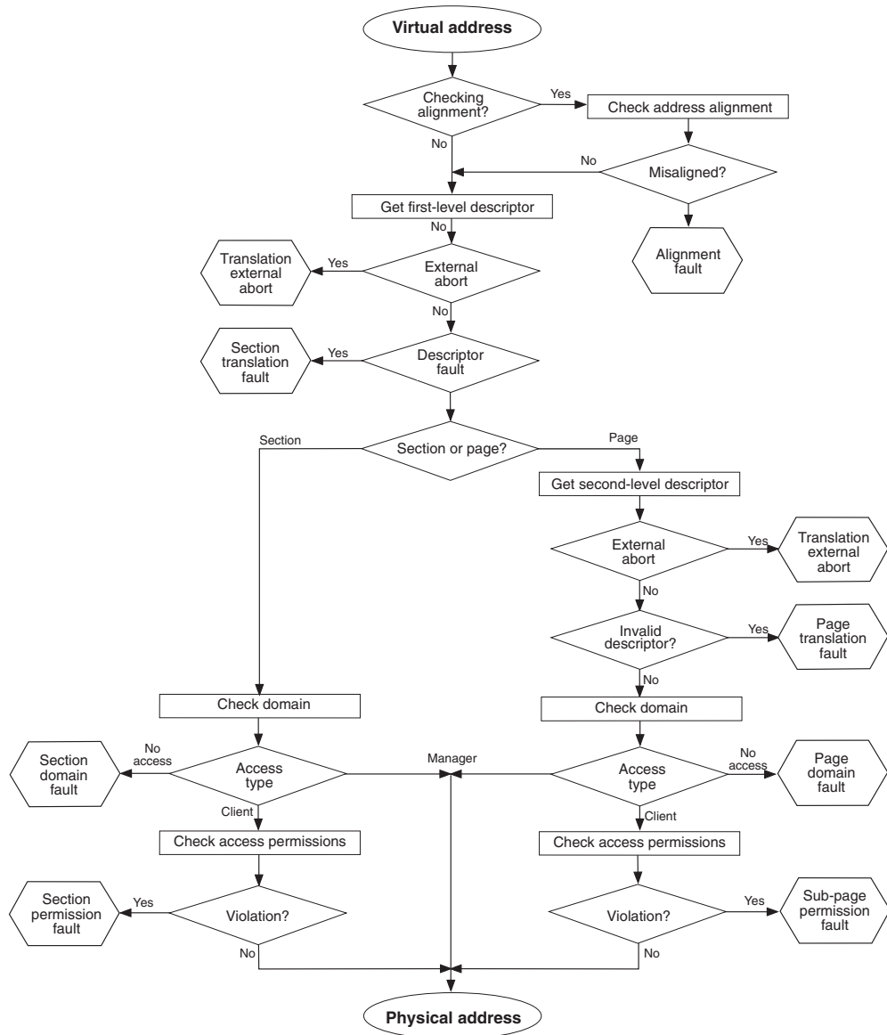
Figure 3-9 Sequence for checking faults
