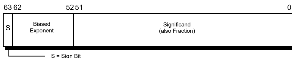
Figure 4-4. Floating-Point Data Types
