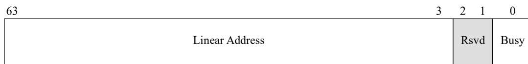
Figure 18-3. Supervisor Shadow Stack Token
