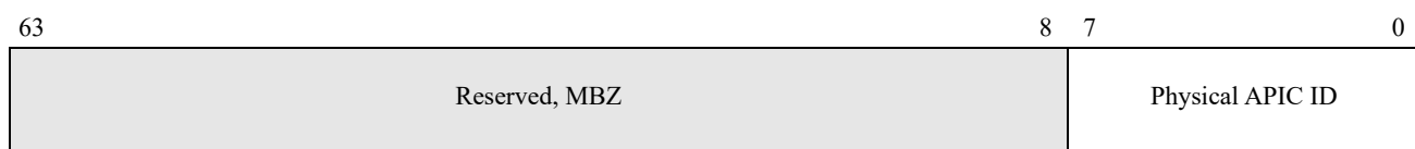
Figure 15-22. Doorbell Register, MSR C001_011Bh
