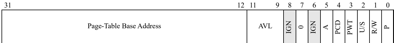
Figure 5-5. 4-Kbyte PDE—Non-PAE Paging Legacy-Mode
