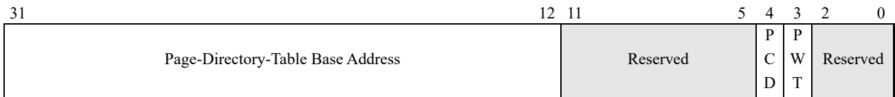
Figure 5-2. Control Register 3 (CR3)—Non-PAE Paging Legacy-Mode
