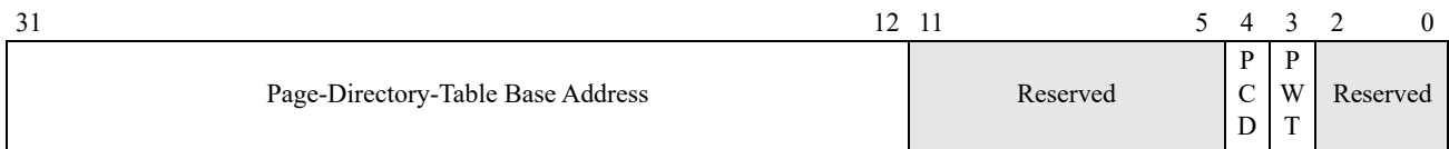
Figure 3-4. Control Register 3 (CR3)—Legacy-Mode Non-PAE Paging
