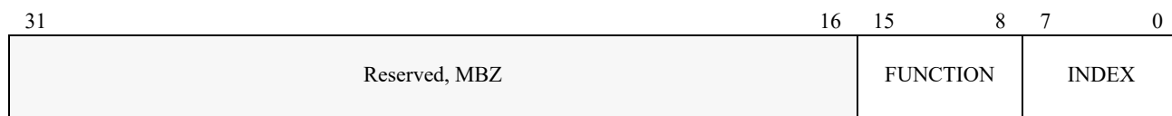
Figure 15-8. Format of DEV_OP Register (in PCI Config Space)
