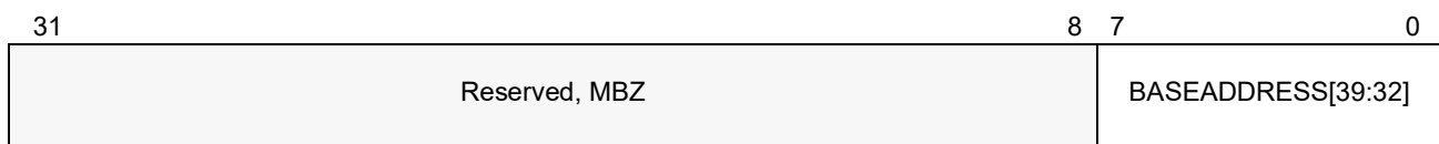
Figure 15-9. Format of DEV_BASE_HI[n] Registers
