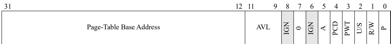
Figure 5-5. 4-Kbyte PDE—Non-PAE Paging Legacy-Mode
