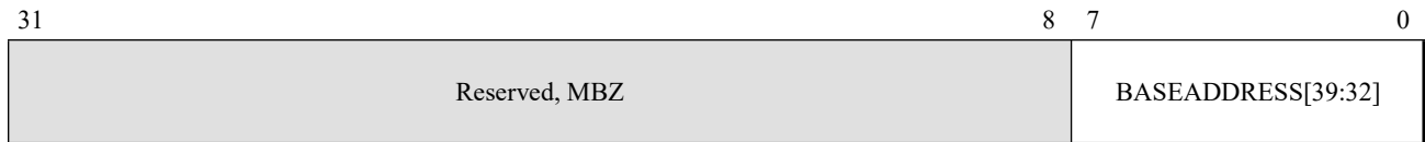
Figure 15-9. Format of DEV_BASE_HI[n] Registers
