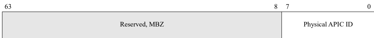
Figure 15-22. Doorbell Register, MSR C001_011Bh
