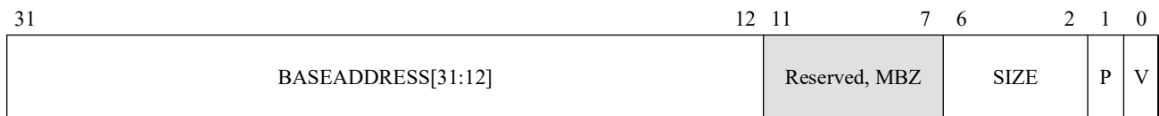
Figure 15-10. Format of DEV_BASE_LO[n] Registers
