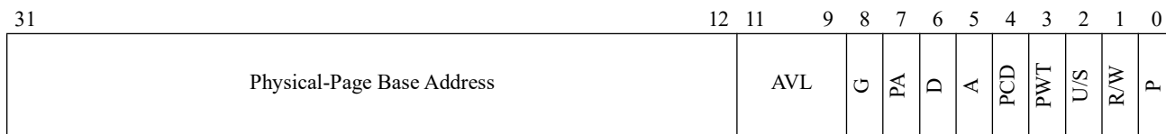
Figure 5-6. 4-Kbyte PTE—Non-PAE Paging Legacy-Mode
