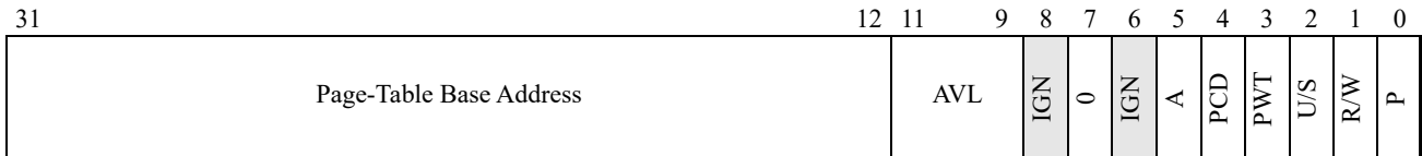
Figure 5-5. 4-Kbyte PDE—Non-PAE Paging Legacy-Mode
