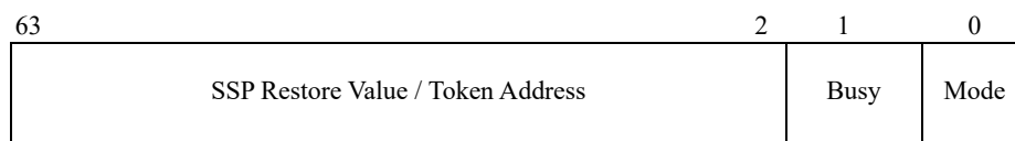
Figure 18-4. Shadow Stack Restore Token
