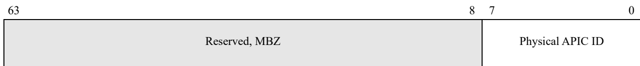
Figure 15-22. Doorbell Register, MSR C001_011Bh
