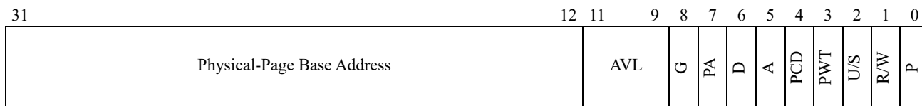
Figure 5-6. 4-Kbyte PTE—Non-PAE Paging Legacy-Mode
