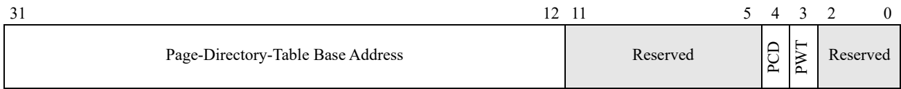
Figure 3-4. Control Register 3 (CR3)—Legacy-Mode Non-PAE Paging
