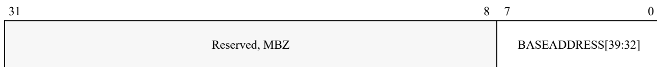
Figure 15-9. Format of DEV_BASE_HI[n] Registers
