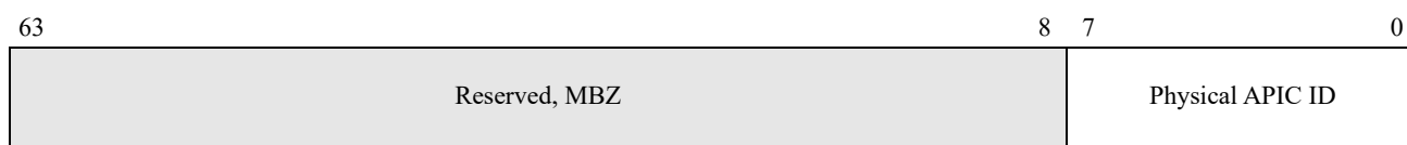
Figure 15-22. Doorbell Register, MSR C001_011Bh
