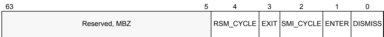
Figure 15-26. Layout of SMM_CTL MSR (C001_0116h)
