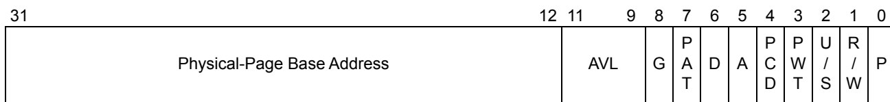
Figure 5-6. 4-Kbyte PTE—Non-PAE Paging Legacy-Mode
