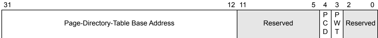
Figure 3-4. Control Register 3 (CR3)—Legacy-Mode Non-PAE Paging
