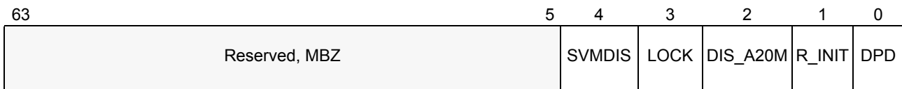
Figure 15-25. Layout of VM_CR MSR (C001_0114h)
