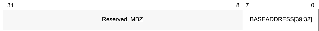
Figure 15-9. Format of DEV_BASE_HI[n] Registers
