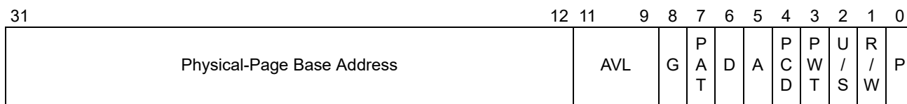
Figure 5-6. 4-Kbyte PTE—Non-PAE Paging Legacy-Mode
