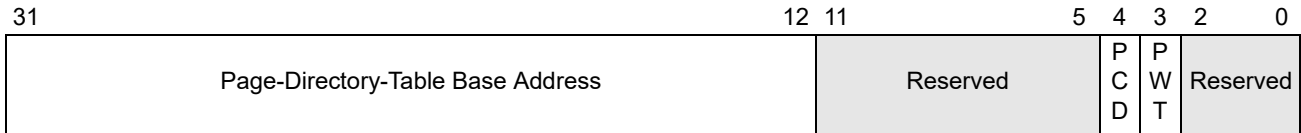
Figure 3-4. Control Register 3 (CR3)—Legacy-Mode Non-PAE Paging
