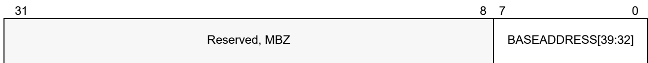
Figure 15-9. Format of DEV_BASE_HI[n] Registers
