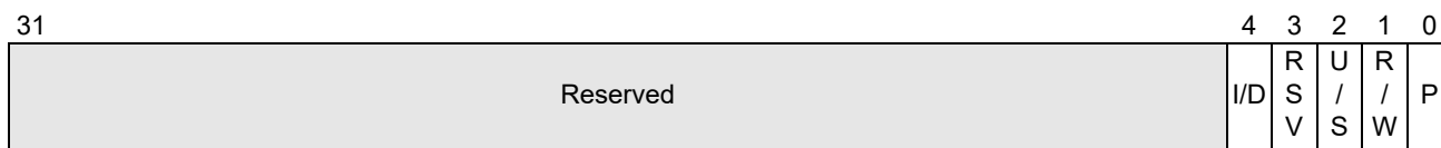
Figure 8-3. Page-Fault Error Code
